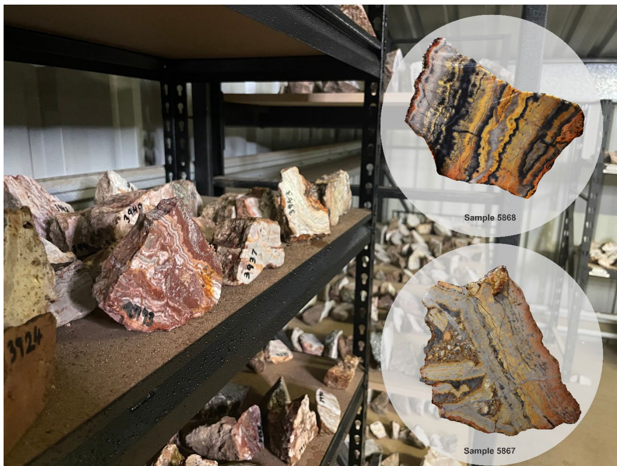
Figure 3: The Bauloora Epithermal Gold Project Rock Library showing an extensive catalogue of surface rock samples obtained and logged during the systematic mapping of the vein field. Surface rock samples 5867 and 5868 show well developed quartz (white-very dark grey)-chalcedony (grey/white)-adularia (yellow-orange) with colloform-crustiform banding and brecciation and an estimated 0 - 5 trace % sulphides 5 and assays pending.
