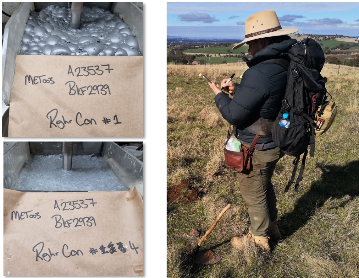
Figure 1: Mt Felstead Prospect rougher flotation concentration stages one and four (BKF2939) and regional soil geochemical sample collection program underway
