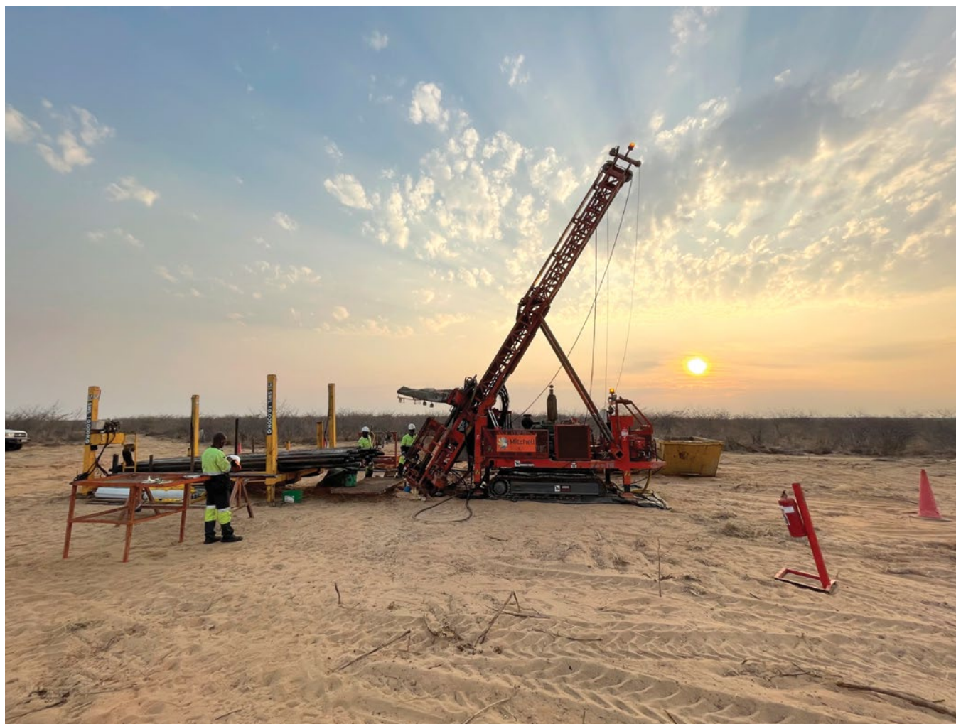
Diamond drilling at the Ngami Copper Project, Botswana
