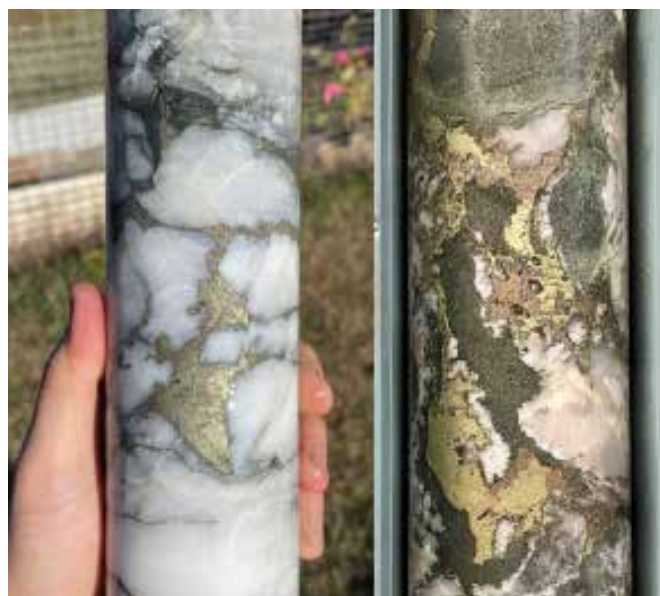
BTDD005 – 699.9m (left), 708.5m (right) – buck quartz vein with chalcopyrite-pyrrhotite infill.
