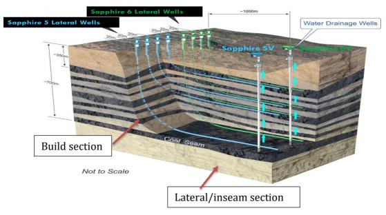
Figure 1: Schematic of Sapphire 5 and 6 pilot well configuration
