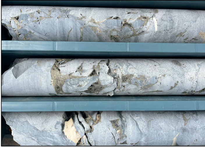
Figure 7. Section of HQ drill core showing cavities with some sulfide infill between breccia fragments. MPD003 HQ3 diameter drill core between 110 and 118m.
