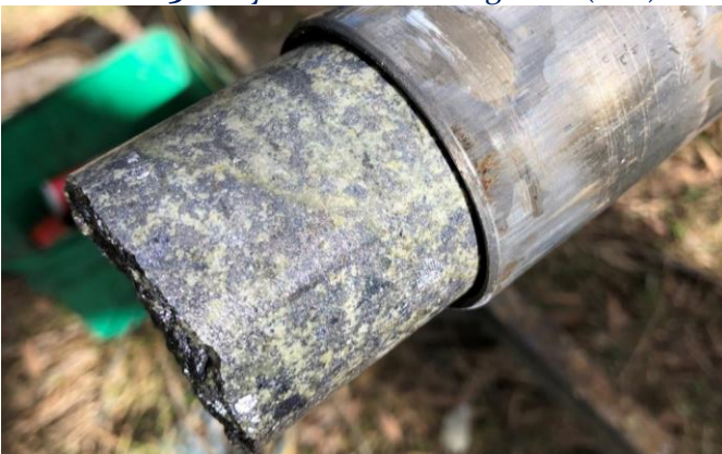
Photos 2 & 3: Very coarse blebs of galena (PbS) in WCS019 drill core (NQ2 core size)
