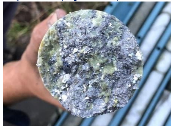
Photos 2 & 3: Very coarse blebs of galena (PbS) in WCS019 drill core (NQ2 core size)
