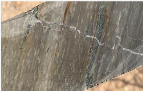
NCP21: Chalcocite and chrysocolla mineralisation at Nova Target
