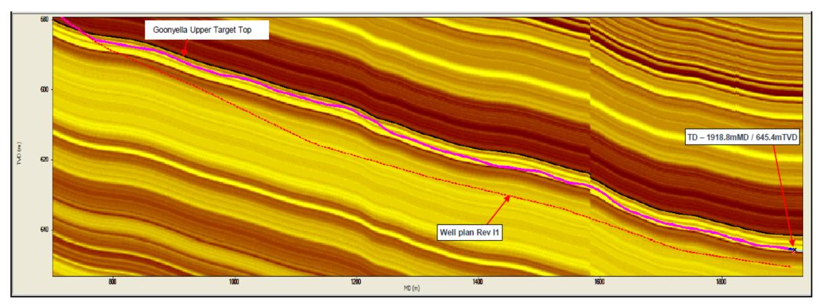
Lateral wells drilled by Sperry using real time gamma imaging tool to hit a 7" target 1.4 kilometres away.
