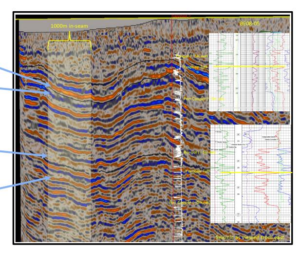
Deepest target seam targeted by L1 Lateral – drilled first for control of shallower targets
