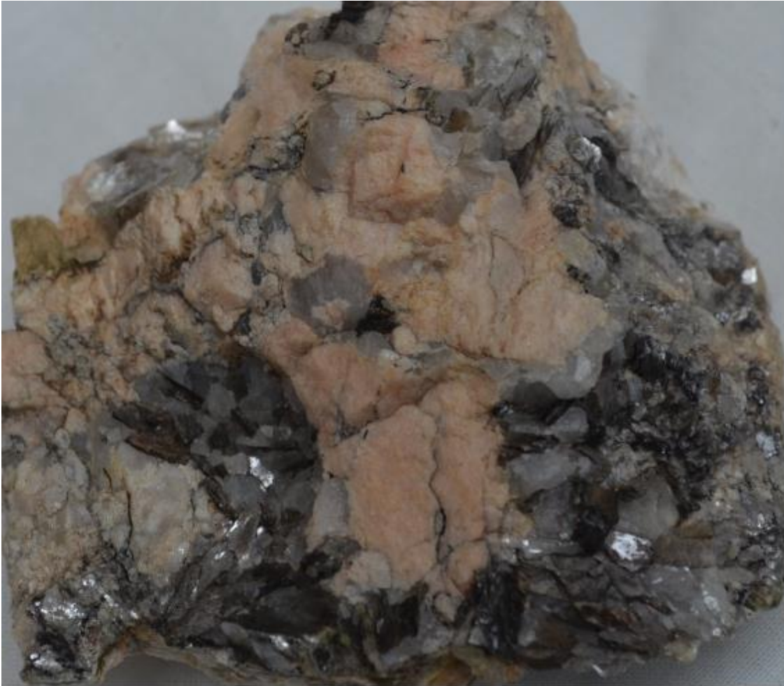
Figure 3: Sample of LCT Pegmatite from historical beryl and tantalum workings (waypoint 1707) (assay results for this sample are yet to be received)* The sample presented in figure 3, is a representative sample of the pegmatites from the Cerro Cora and Porta D'Agua tenements. It comprises primarily of quartz, orthoclase feldspar, tourmaline and micas. No visible spodumene was observed in the sample.
