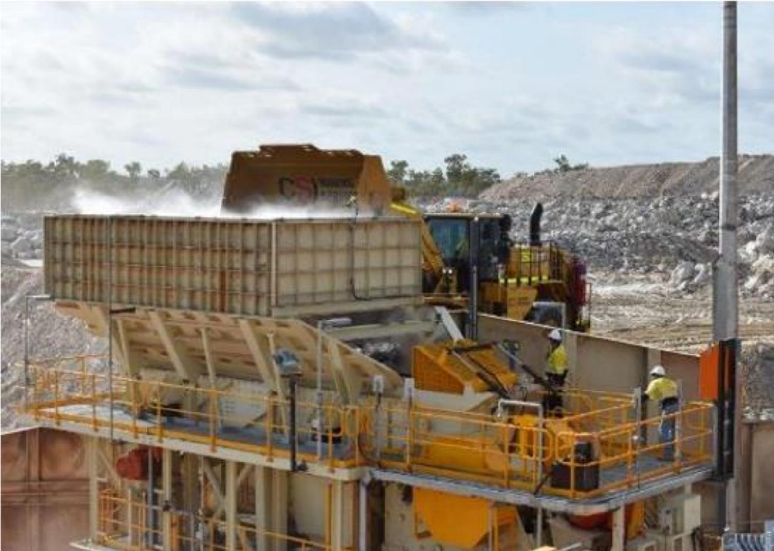
Loading the crushing plant
