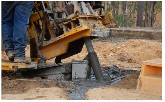
By XRF sampling the water return line on the drill rig we can quickly see indicators which have excellent correlation to lab assay results (lab assay left sludges right on adjacent figure) providing confidence to proceed without waiting for the lab.
