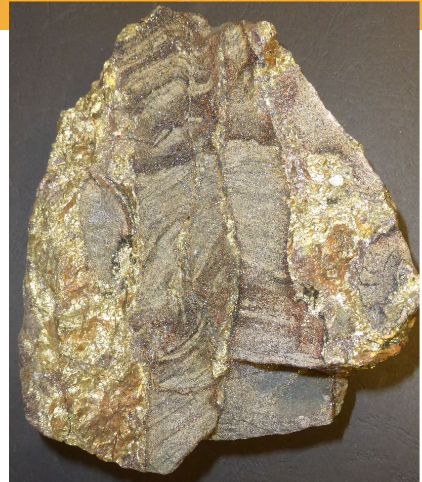
Garnets/andalusites depict the bedded layers, which are truncated by veins infilled with Cpy and Po
