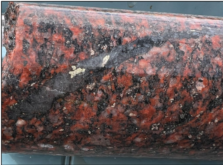
Figure 16. Image showing quartz vein cutting across sericite and hematite altered host granite. The vein contains pyrite and magnetite and is similar to pyrite-magnetite-quartz veins observed around the Olympic Dam IOCG deposit.
