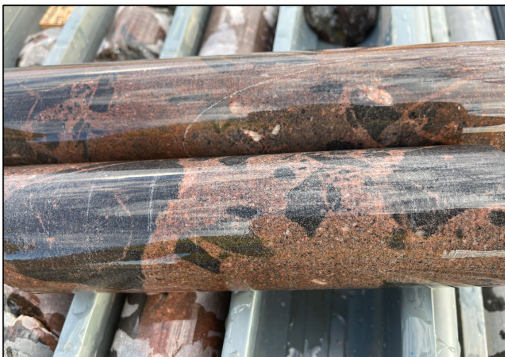
Figure 14. Image fo NQ 1/2 drill core HELIOS_DD02 showing the bimodal mafic (black) igneous rocks mingling with felsic (pale pink) host granitic rocks. The granite is partly altered and locally porphyritic with well-defined potassium feldspar phenocrysts. The textures presented in this sample are indicative of co-mingling between mafic and felsic rocks near the margin of a larger mafic intrusive.
