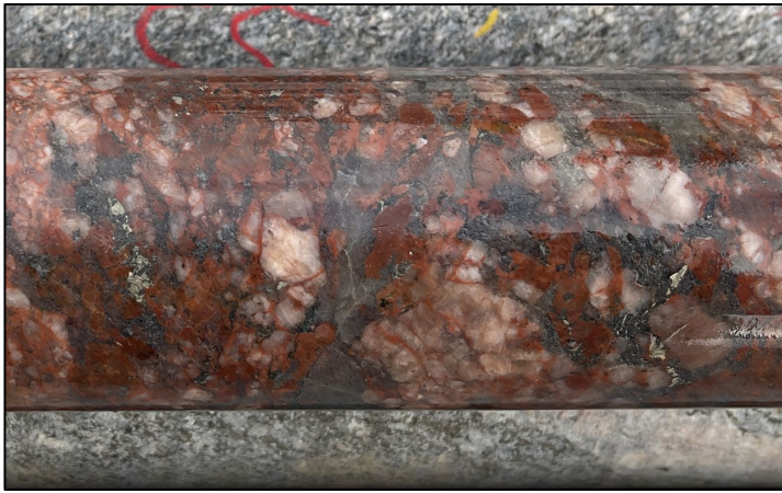
Figure 11. Image fo NQ drill core HELIOS_DD01 showing heavily hematite stained granite breccia together with hematite, pyrite and minor quartz replacement of groundmass
