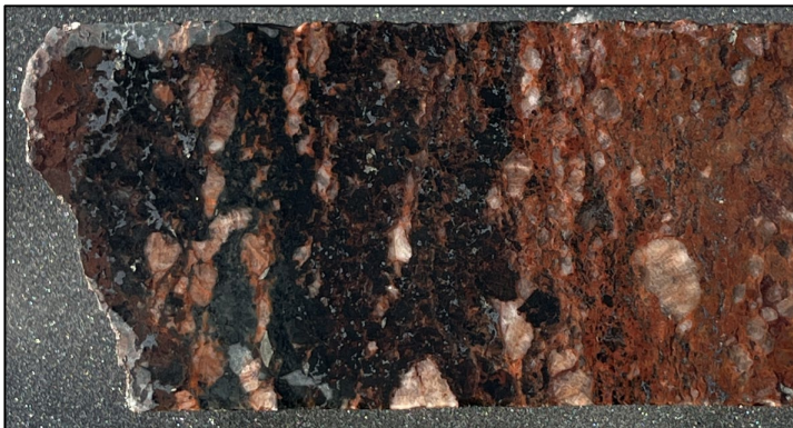
Figure 13. Image fo NQ 1/2 drill core HELIOS_DD01 showing a range of alteration minerals and textures. Red alteration is hematite staining of host granite and replacement of groundmass. Part of the rock is also replaced by biotite, amphibole and hematite. The host granite is almost unrecognisable in this part of the drill core due to the pervasive multi-phase alteration.
