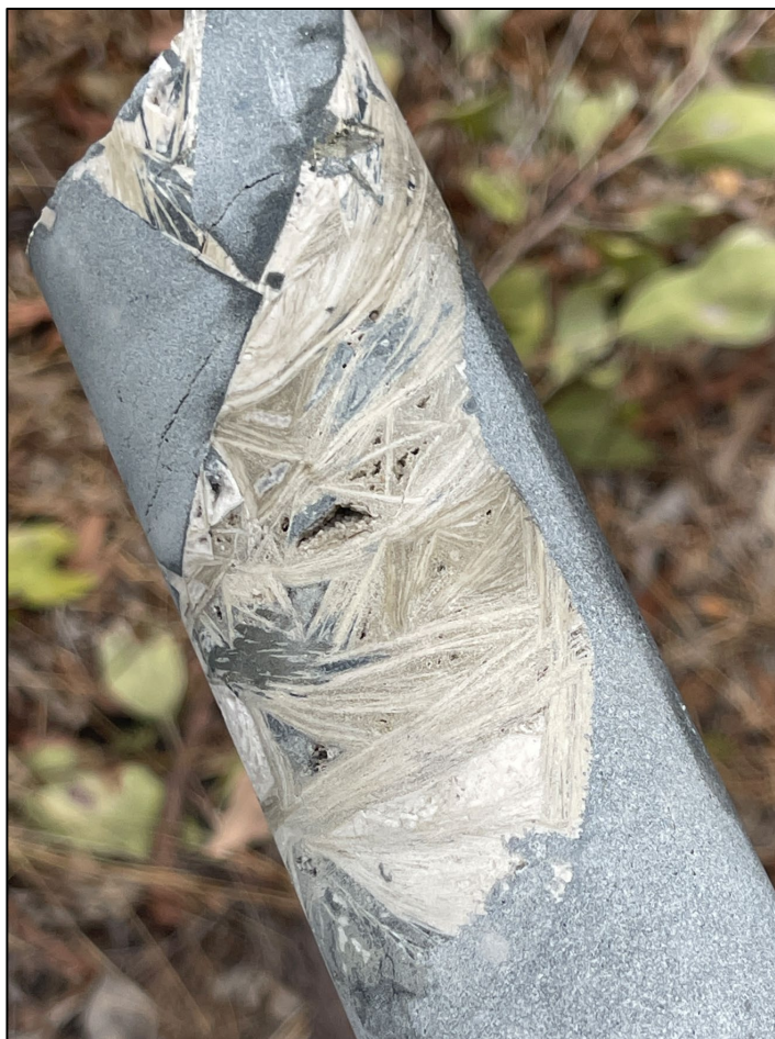
Figure 4. Section of ØNQ drill core from MPD003 (183.4m) containing wollastonite and sphalerite+pyrite between metamorphosed and altered host sandstones (meta-sandstone protolith). Wollastonite is ( \text{CaSiO}_3 ) a good indicator mineral for skarn-type mineral deposits including the nearby Chillagoe deposits (e.g. Redcap) where Wollastonite forms part of a prograde skarn assemblage.
