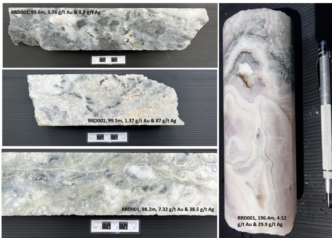
Figure 9: RRD001 drill core photos showing examples of multiphase quartz veins and presence of disseminated and thinly banded grey sulphide minerals. Vertical core specimen at right shows colloform banded quartz with pale amethyst.
