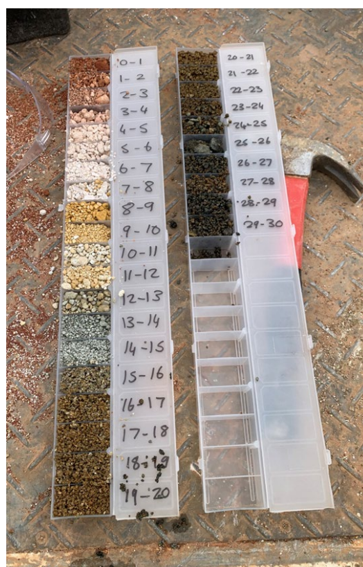
Photo: Typical weathered profile (Meteor Prospect) - red-brown transported cover from 0 to 4m, then white and coloured saprolite clay, transitioning to saprock from 15 metres and finally fresher basement rock from 28 metres.
