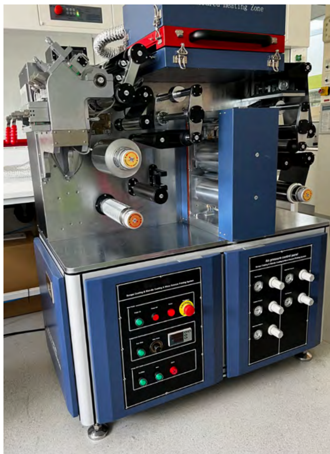
Phase 2 includes two roll-to-roll cathode coaters that precisely coat our unique cathode materials onto aluminium foil.
