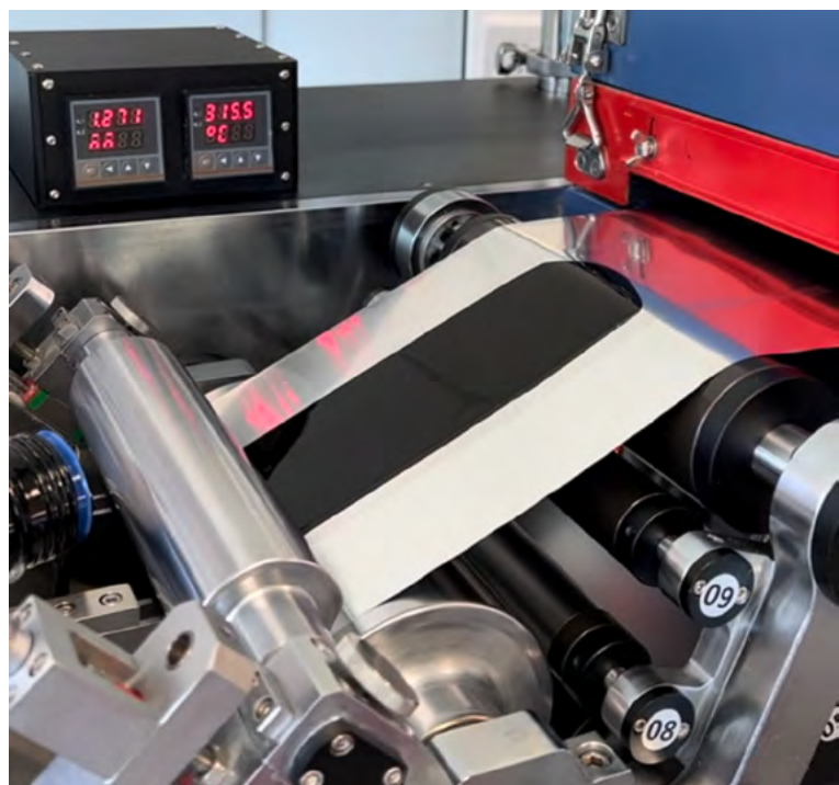
The wet coated cathode then enters the drying ovens before completing the coating process.
