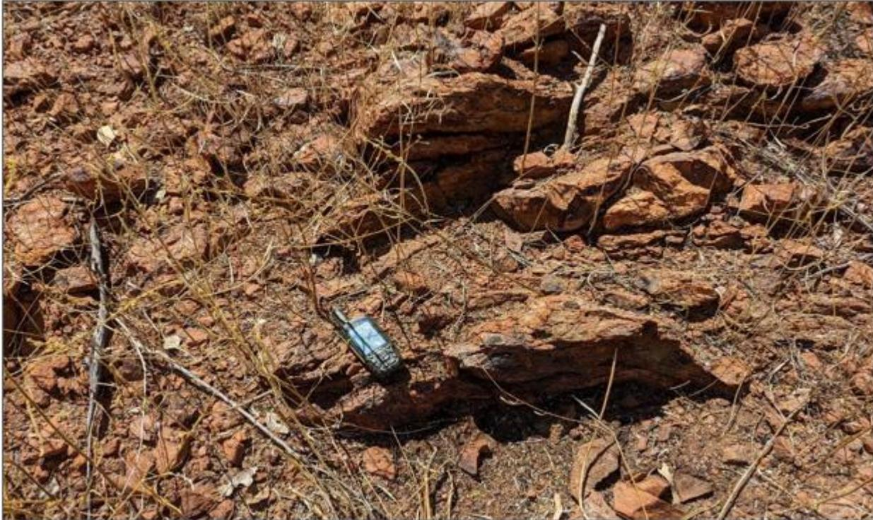
Figure 6; Marlin sample location GCM0032 (3.37% TGC) showing outcrop of ferruginous ironstone and graphite.
