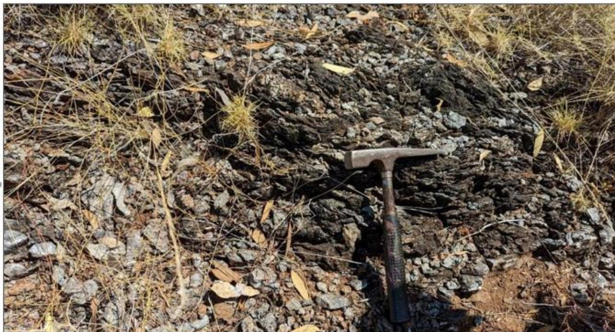
Figure 5; Close up view of graphite outcrop at sample location GCM0010 (2.09% TGC).
