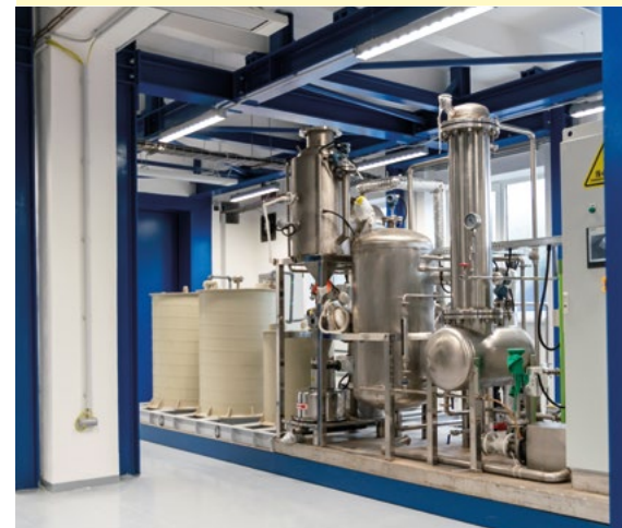
Image: HPMSM crystallization module at the newly installed Demonstration Plant.
