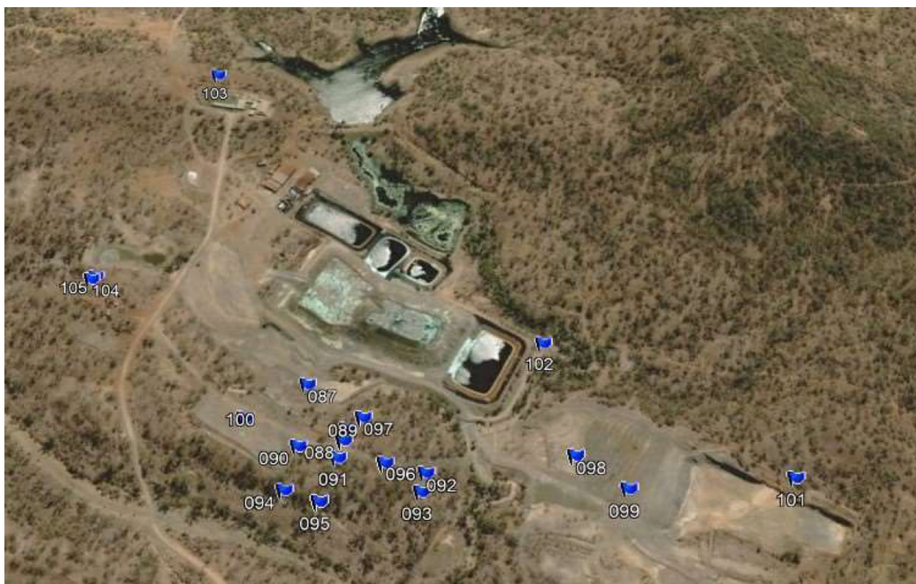
Figure 1. Collar locations for the northern oxide copper zone and the primary (chalcopyrite) copper drilling in the open pit.
