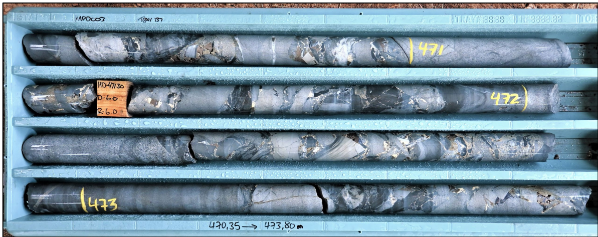
Figure 11. Representative section of brecciated core from MPD003 showing both sandy units (lighter greys) and mud-rich units (dark grey). The host low-grade metasediments are heavily brecciated and show infill with predominantly quartz and carbonate together with sulfides, mainly pyrite with sphalerite and minor galena in MPD003. The metasediments also exhibit fine network veining with sulfides as well as disseminated sulfides throughout. Core is NQ from 470.35m to 473.8m down hole. The average silver grade is 10g/t Au from sample MPDN470 (470-471m) to sample MPDN473 (473-474m).
