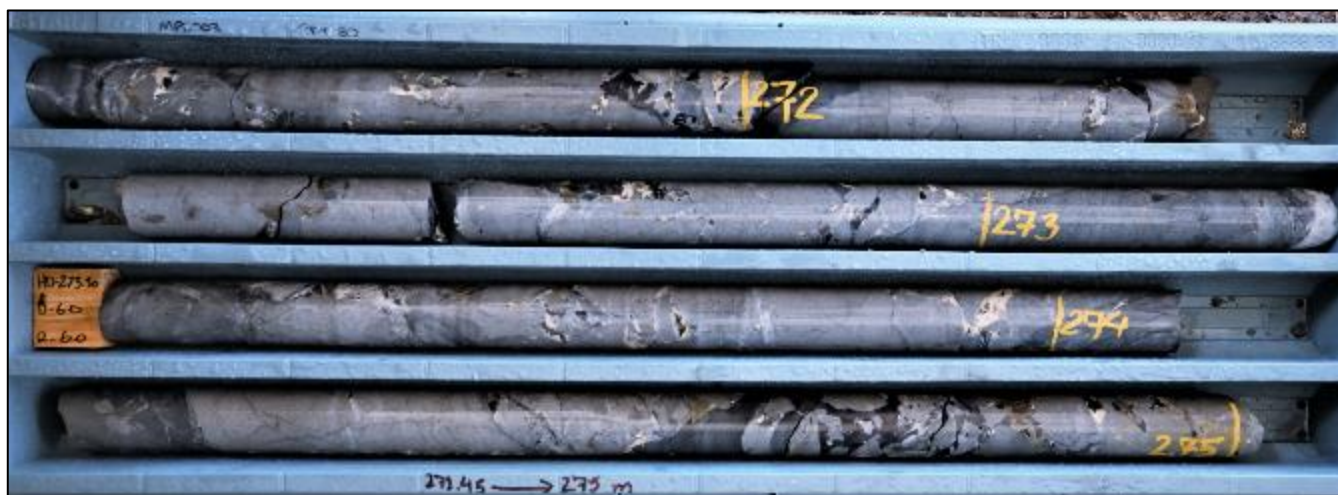
Figure 1. Section of drill core from 271.45-275m with assay results for 271m-275m (5m) containing 37.1 g/t Ag, 2.8 % Zn, 0.52% Pb and 212g/t Sb.
