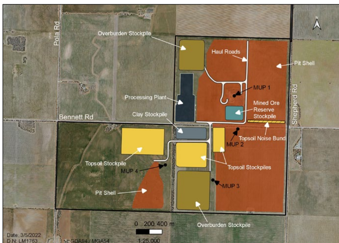
Figure 18: Area 1 surface infrastructure
