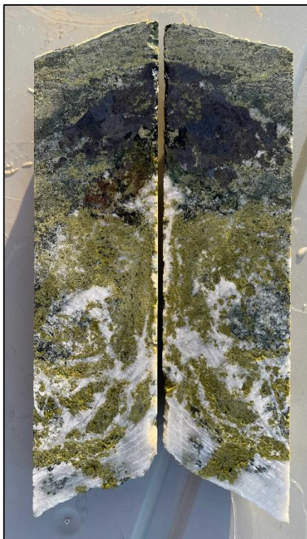
Figure 10: EVDD2203 – 20m - Sphalerite mineralisation hosted by carbonate – epidote calc silicate
