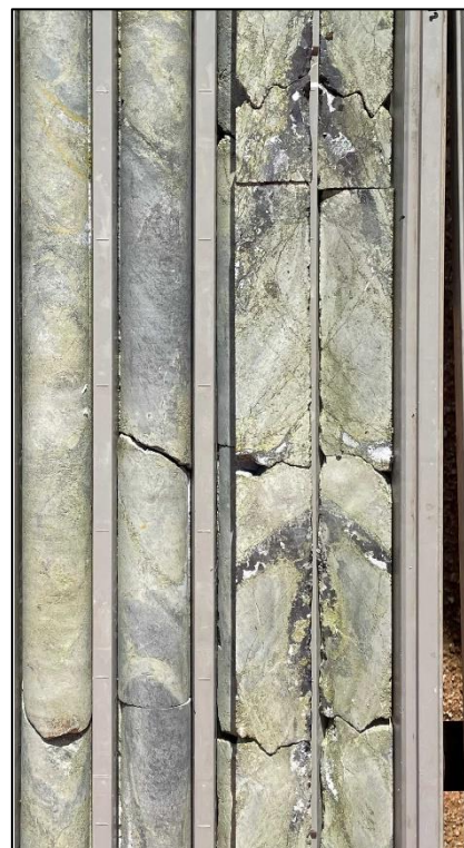
Figure 12: EVDD2203 – 38m - Sphalerite developed on structures in meta basalt breccia?
