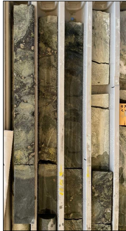
Figure 11: EVDD2203 – 101m - Breccia infill mineralisation
