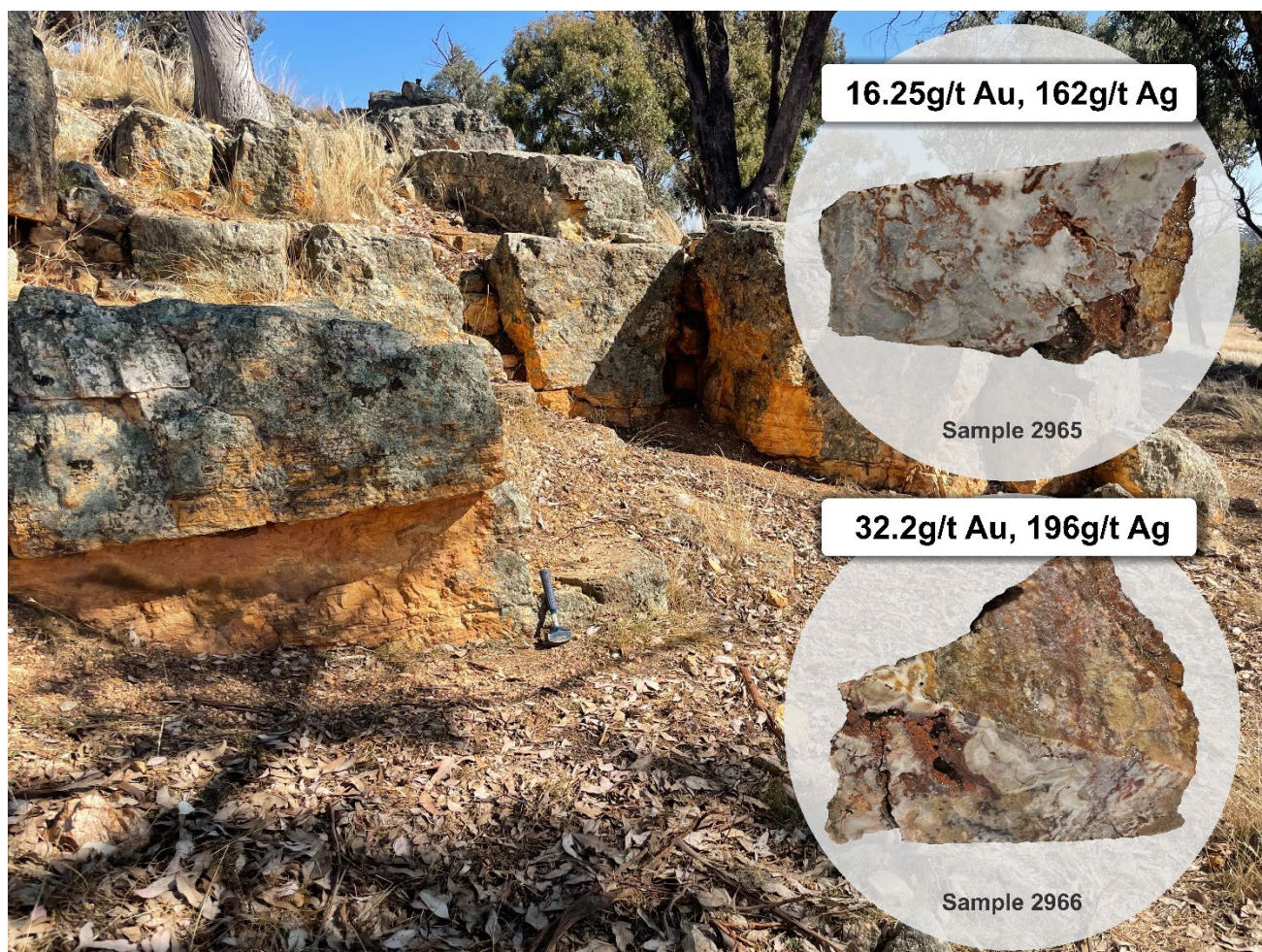
Figure 3: Outcropping sinter lithology 2 at the Breccia Sinter Prospect and rock chip sample 2965 showing hydrothermal breccia with suspected hypogene hematite and crustiform-colloform chalcedony-quartz vein and 2966 showing hydrothermal breccia with suspected hypogene hematite and crustiform-colloform chalcedony-quartz vein 3
