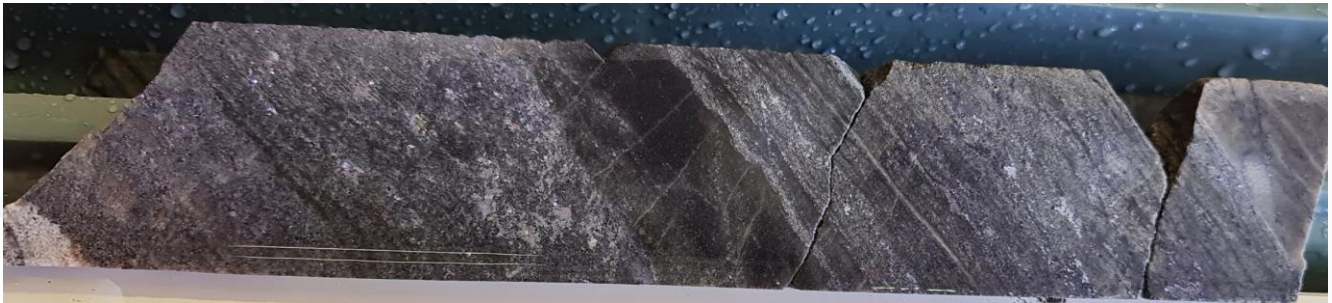
[Figure 1] Image of half core showing strong galena mineralisation at 1295m downhole from within the Western Horizon
