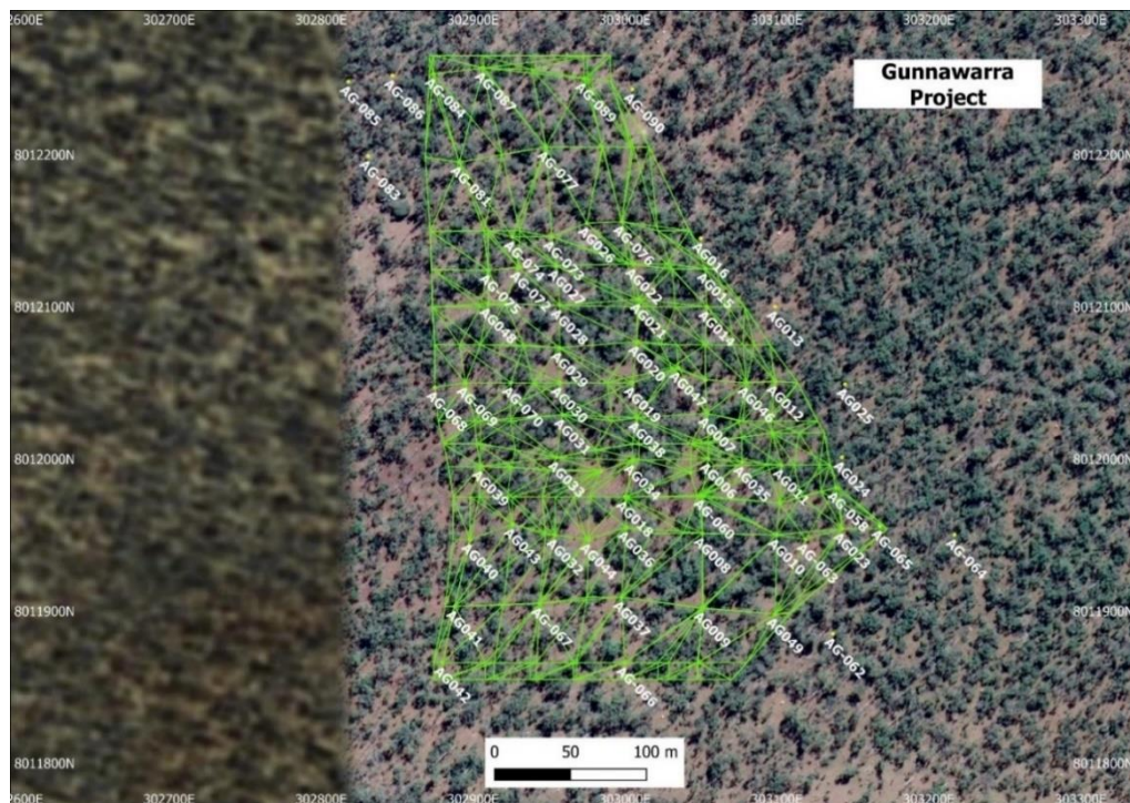
Figure 2: Drill hole collar plan with interpretation wireframe. This shows the hole numbers and locations. The wirelines link the resource material together.
