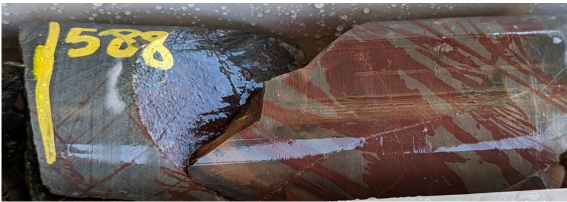
Figure 8. 'Bleed' textured hematite alteration of siltstone (588m).
