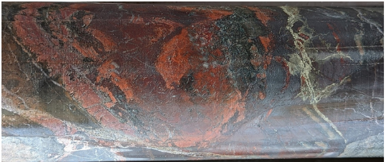
Figure 9. Pyrite vein cutting hematitic ironstone (663.8m).
