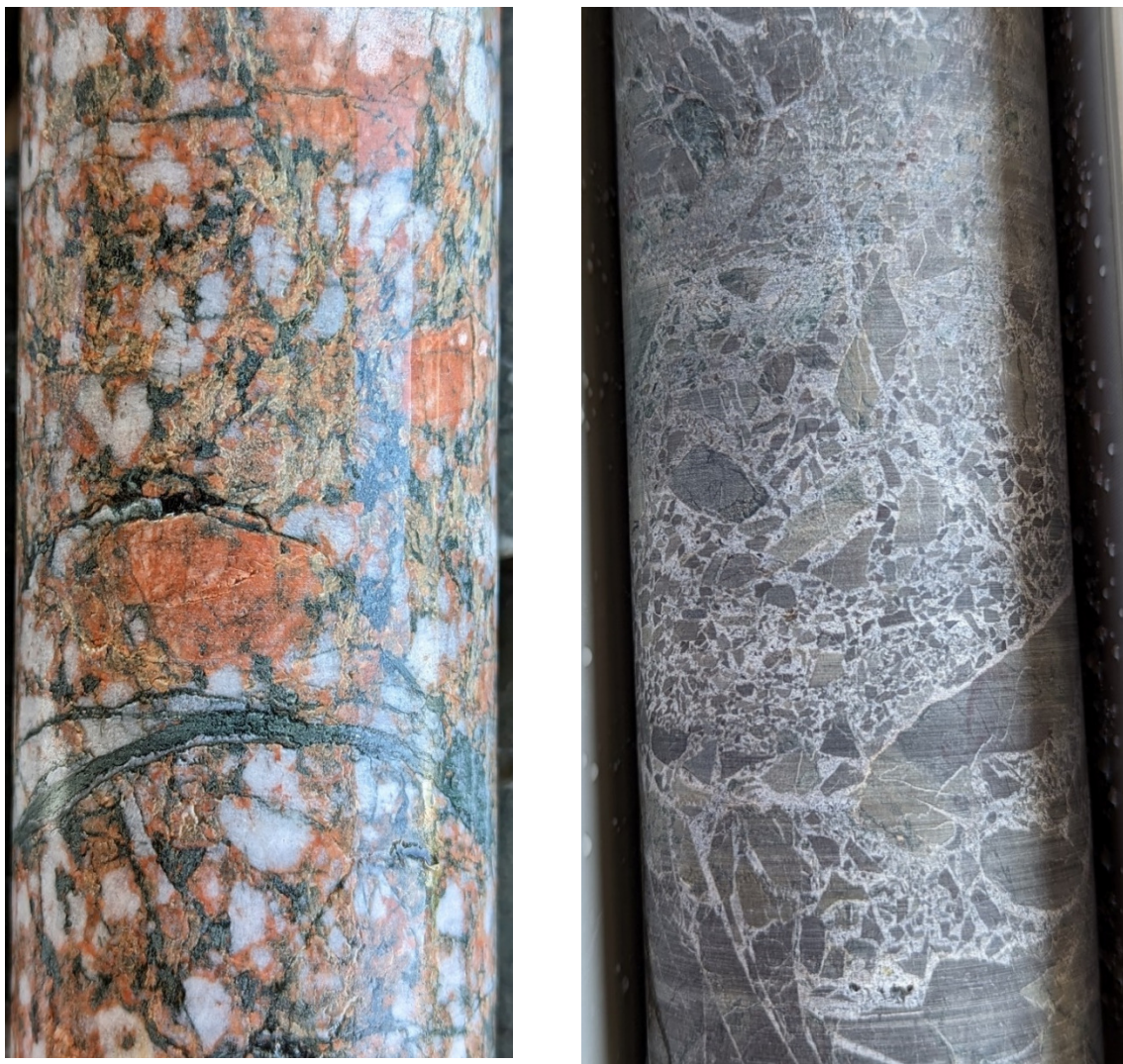
Figure 4. Coarse-grained granite (left, 247.7m) and brecciated siltstone (right, 581.5m).
