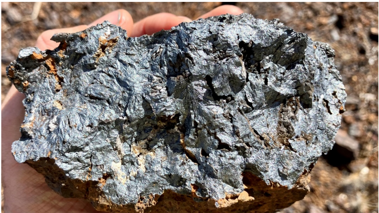
Figure 9. Manganite sample showing pyrolusite needles (Sample#ZEU110).
