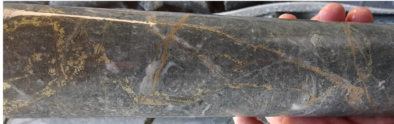
Chalcopyrite stockwork veining overprinting secondary biotite (potassic altered) diorite porphyry
