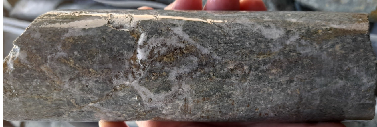
Chalcopyrite dominant stockwork veining and quartz-chalcopyrite breccia veining overprinting secondary biotite (potassic altered) diorite porphyry
