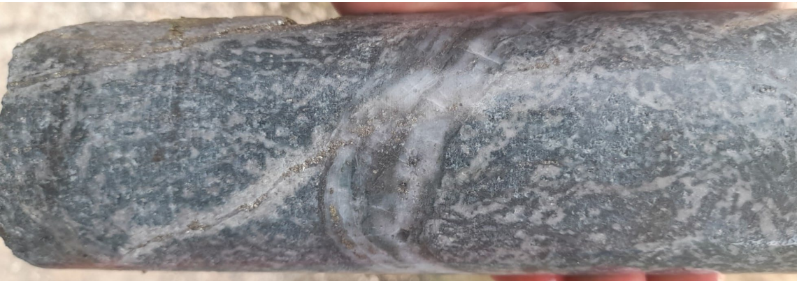
Porphyry B-veins with chalcopyrite-pyrite sulphide mineralization cut by late porphyry pyrite D-vein with sericite (phyllic) selvage
