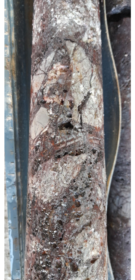
Porphyry B-veins and breccias with abundant iron-oxides (after sulphides) preserved in oxide gold zone
