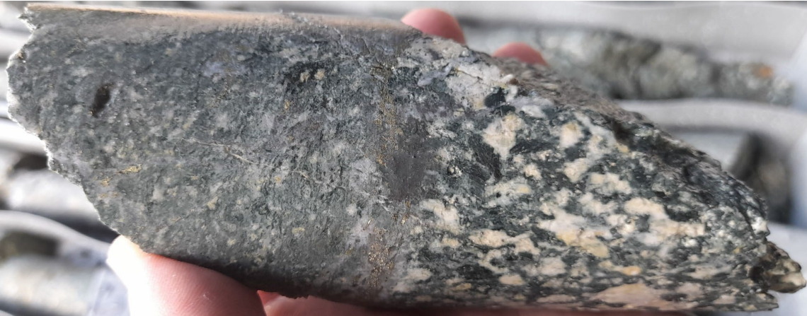
Intrusive contact between diorite porphyry with chalcopyrite mineralization (left) and mafic tuff hostrocks (right)
