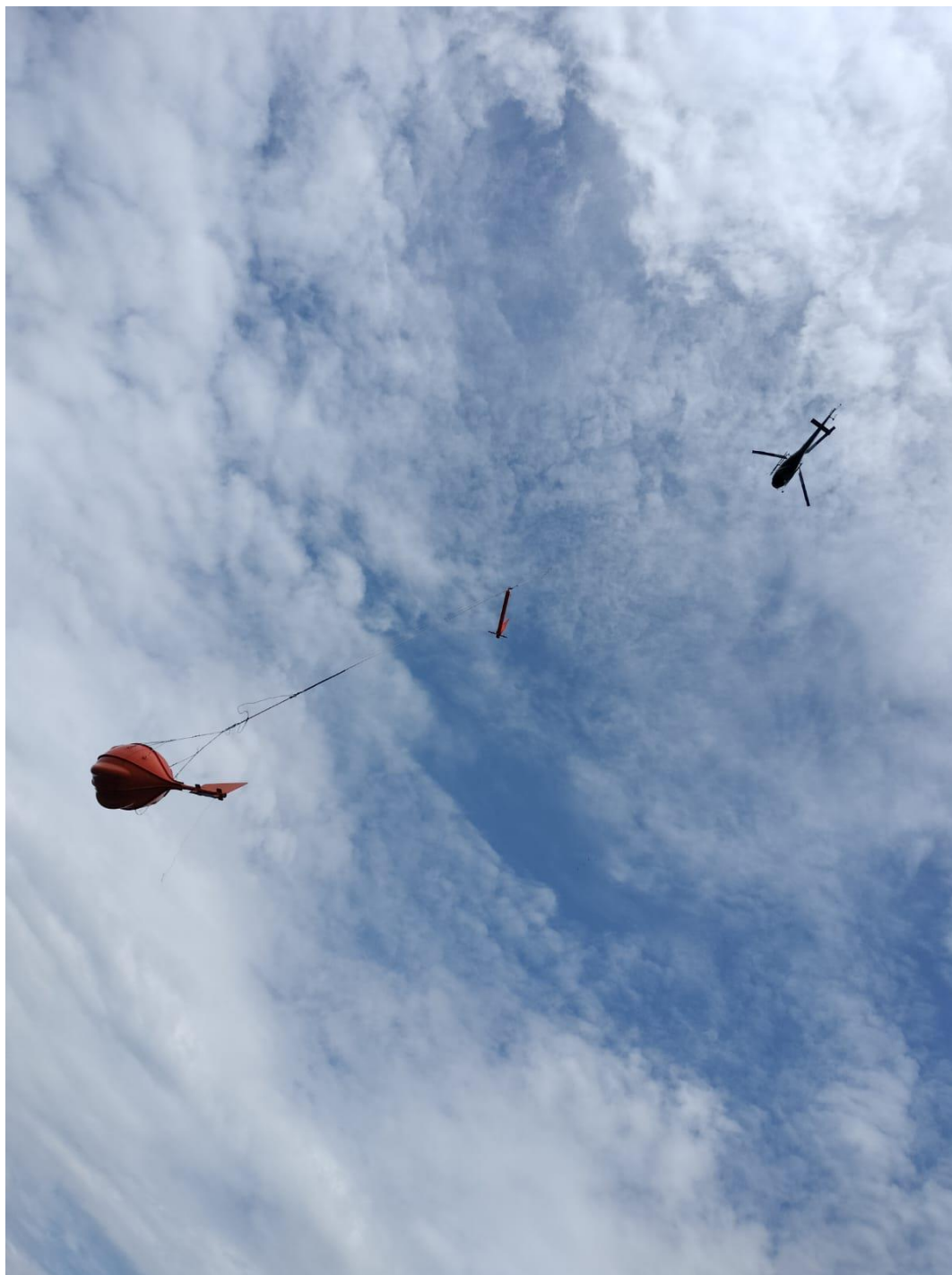
Figure 2: Expert Geophysics Ltd towed bird acquiring MobileMT data in the survey along the Ngongo-Yoyo Trend – December 2022.
