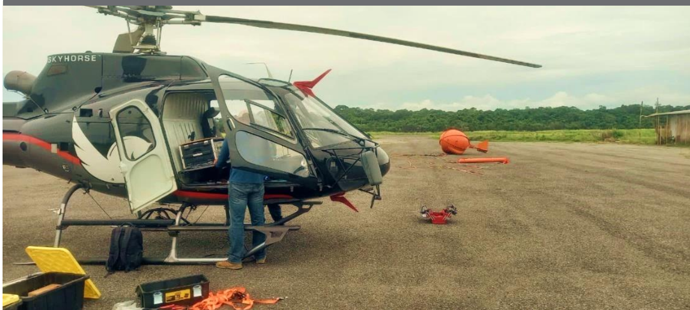
Figures 6: Skyhorse Aviation (Pty) Ltd ('SHA') helicopter (ZS-RSS) with the Expert Geophysics Limited MobileMT system – calibration flight set-up at the Mayumba regional airport.
