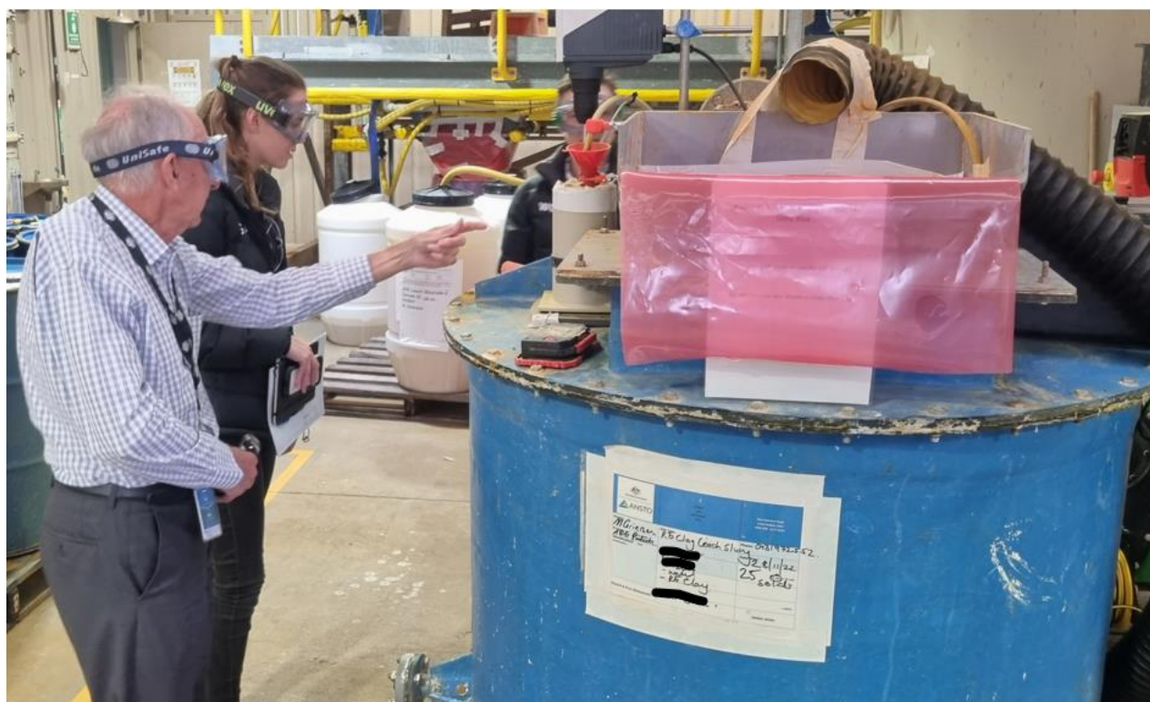
Image 1: Tank based, clay slurry desorption and leaching at ambient temperatures and pressures, for rare earth carbonate production testing from Koppamurra samples at ANSTO under Dr. Bob Ring's supervision.
