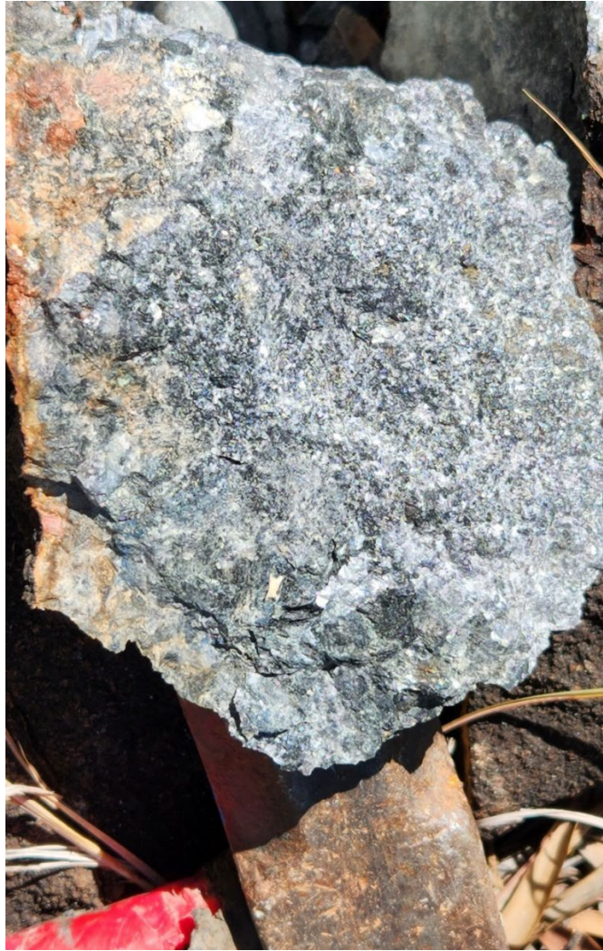
Figure 8. Rock chip of gabbro outcrop taken from Phantom intrusion carrying fine disseminated sulphides.
