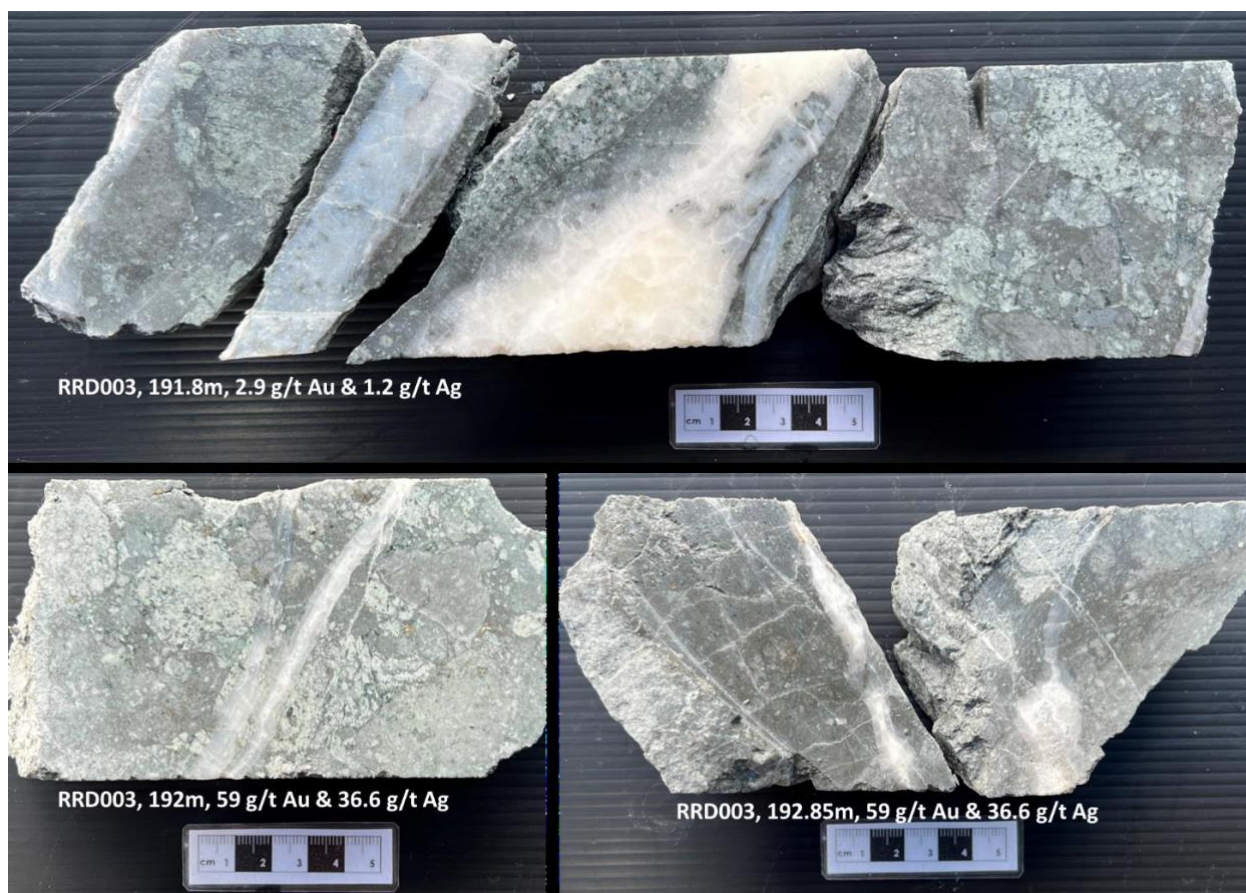
Figure 13: Core photos from deep gold intersection in RRD003. TOP: massive crystalline quartz vein with possibly later opaline blue quartz veins at margin. BOTTOM: high grade Au assay associated with the occurrence of narrow thinly banded crustiform quartz veins.
