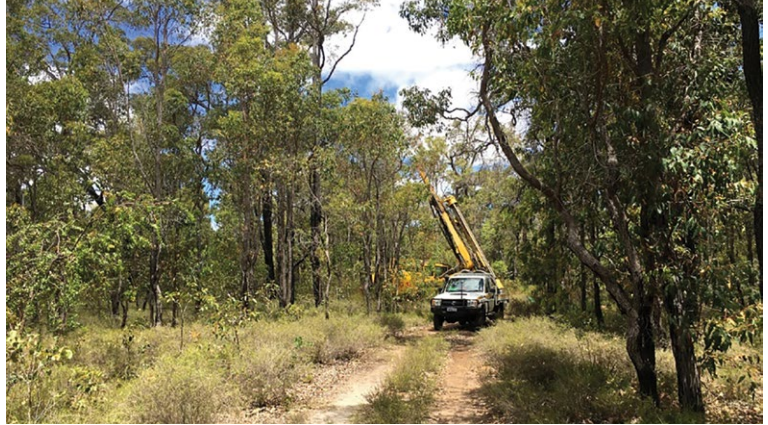
Figure 5: RC drilling underway on an existing track at the East Kirup Lithium Prospect
