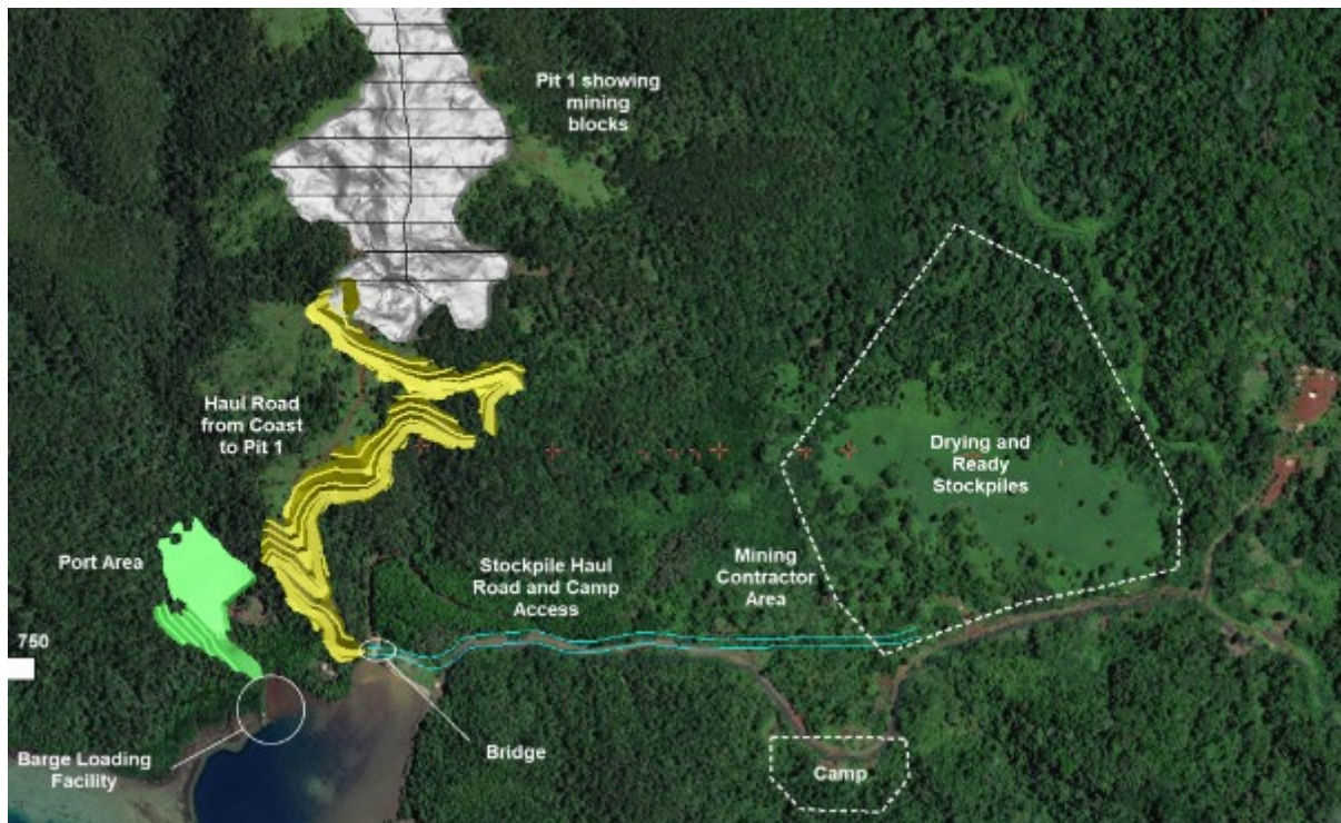
Figure 28 Mine and Operations Site Layout
