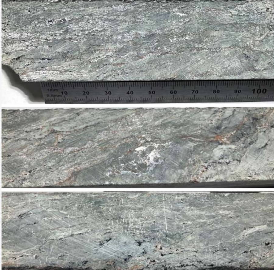
Figure: High-grade chalcocite (silver-black metallic mineral) from drill hole NCP20A. The displayed drill core is grading at 10.9% Cu and 45 g/t Ag. This zone marks the base of the mineralised section and extends for 1.7m downhole.
