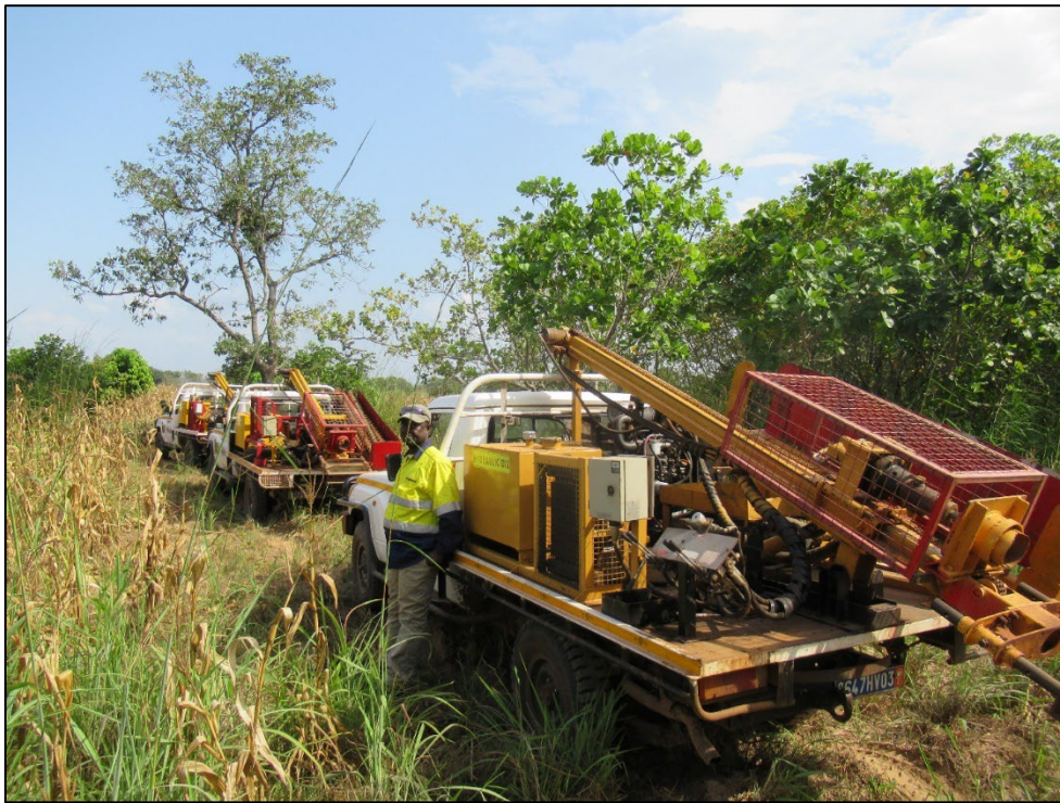
Figure 1 Three of five of auger rigs to be used for infill program
