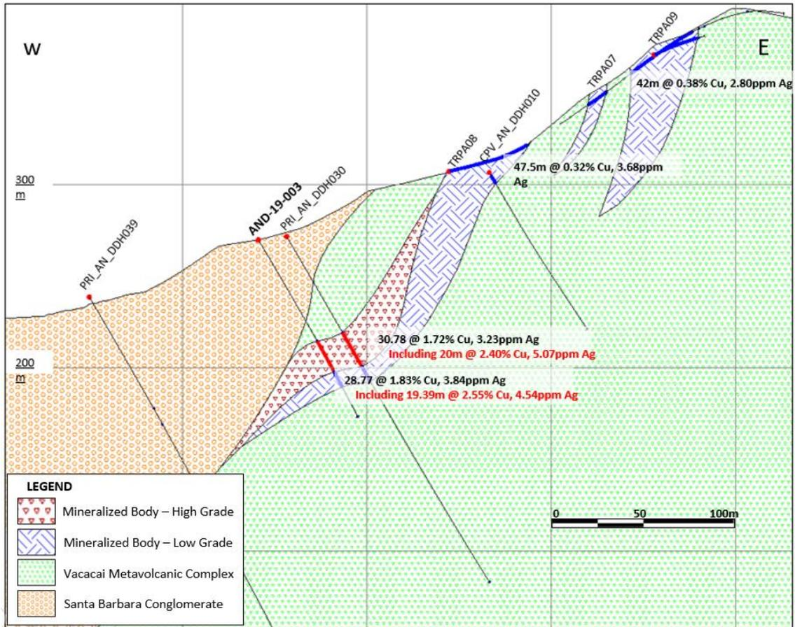
**Figure 5-2 – Representative Drillhole and Geological Vertical Cross Section.**
