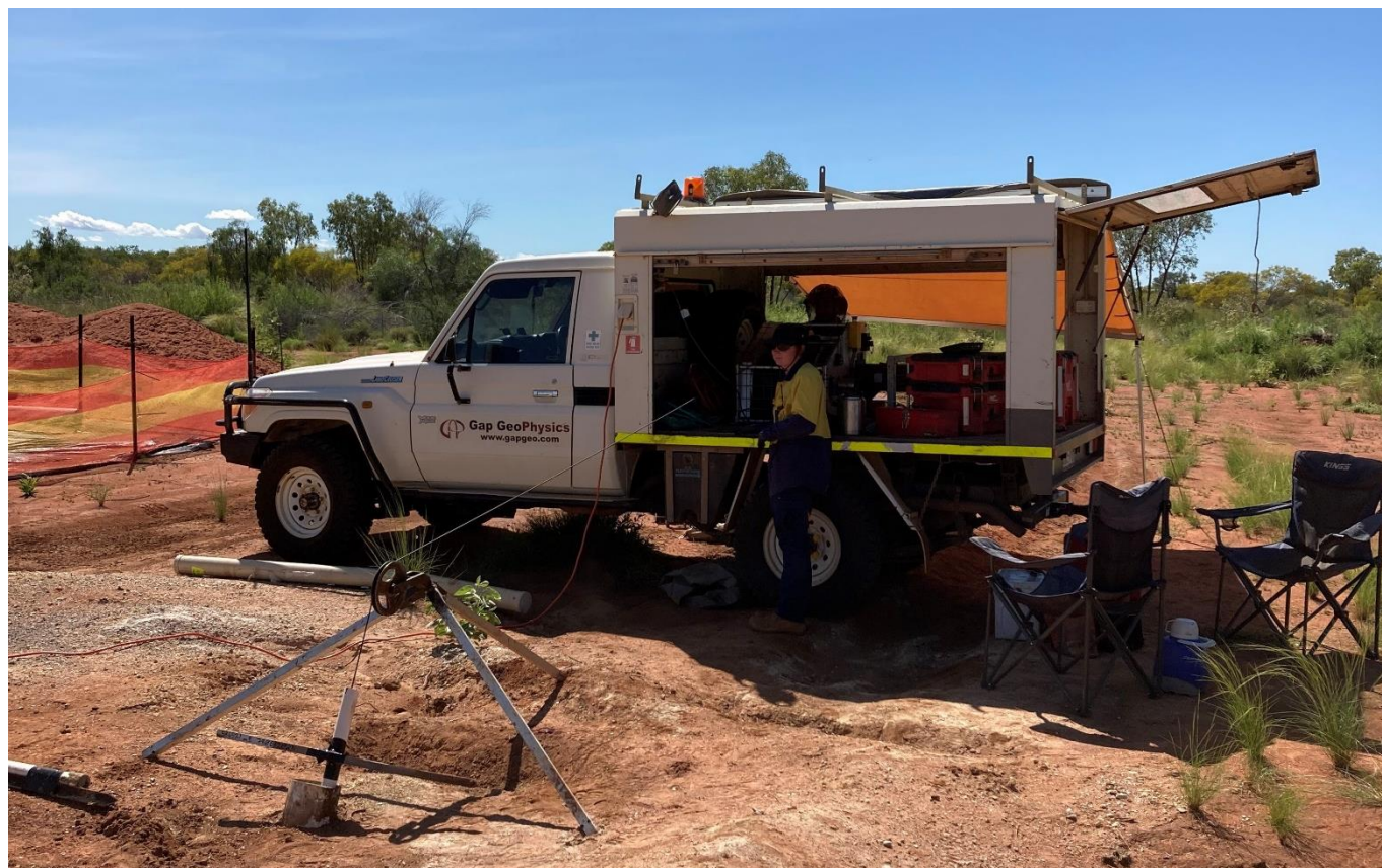
Figure 2. Gap Geophysics conducting downhole surveying on Leichhardt East drillhole KNXLE001RDD.
