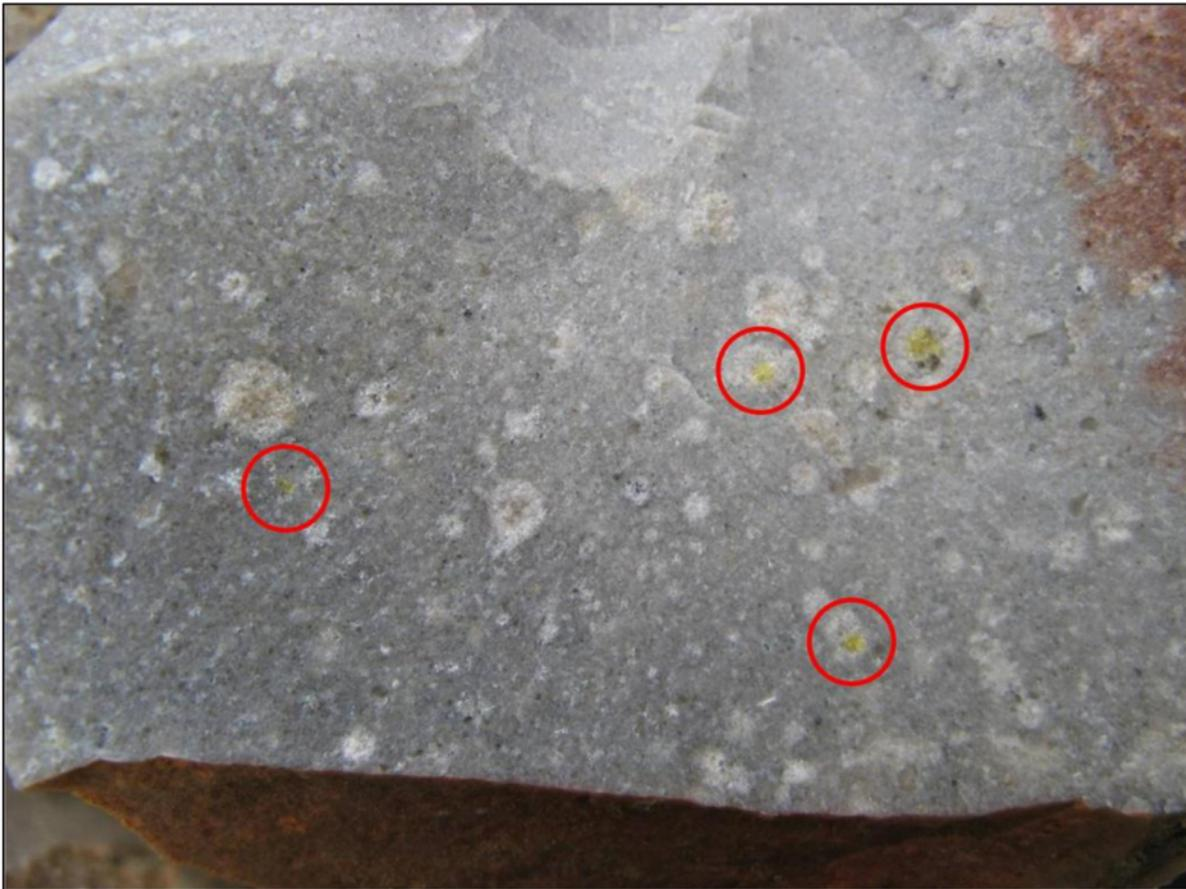
*Figure 5. <sup>1</sup>Carnotite in silicified sandstone. Red circles are ~5mm in diameter (Regalpoint Resources Prospectus, 2011).*
