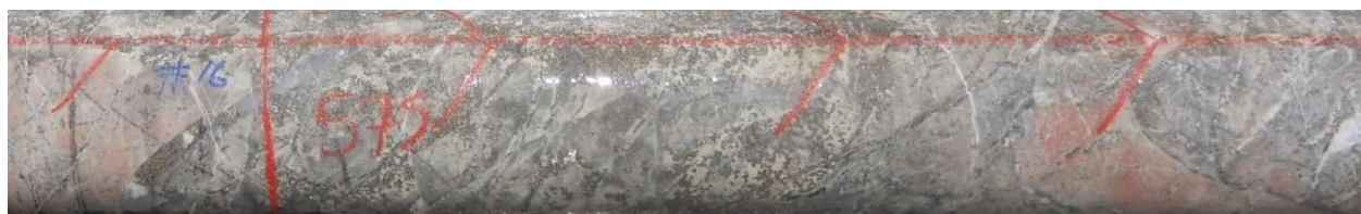
Fig 14. Hole 16, 575m, Close packed, highly sulphidic, clast supported breccia dominated by angular clasts hornfels, -minor altered porphyry. Abundant infill and disseminated pyrite & infill quartz. 574m-575m : 1m @ 0.07% Cu, 0.03 g/t Au, 1 g/t Ag, 11.39% S.
