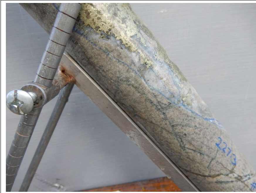
Fig 9 .Hole #16 , oriented in core oriented frame, hole drilling to south, inclined at 55 degrees view looking east. 227.3m : semi-massive quartz pyrite chalcopyrite vein cutting sericite altered diorite dominated hydrothermal breccia. Large diorite clast at bottom cut by early multi-directional quartz sulphide “porphyry-style” stockwork. 227m to 228m : 1m @ 2.56% Cu, 0.41 g/t Au, 42.7 g/t Ag, 5.59%S.
