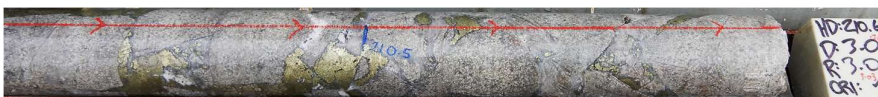
Hydrothermal infill breccia ,altered diorite clasts , chalcopyrite -pyrite -calcite-quartz infill .CAE hole # 16, : 210m-211m depth. 1m @ 2.74% Cu,0.43 g/t Au,71.6 g/t Ag,
