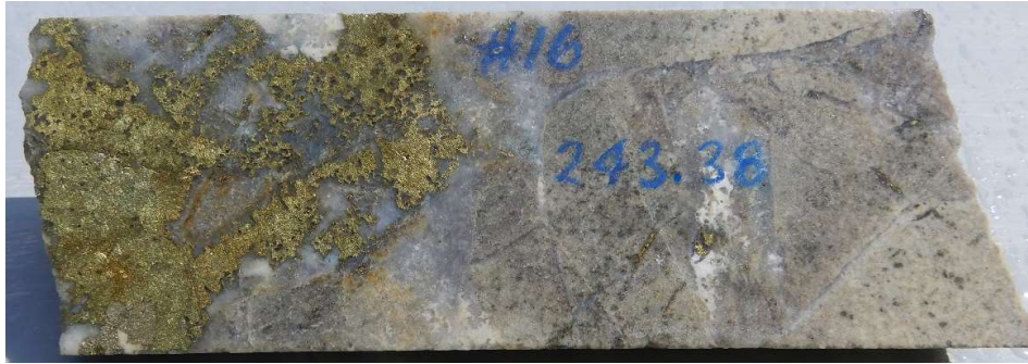
Figs 6 Photo full HQ core Hole #16 , Hydrothermal breccia ,diorite clasts, infill quartz, calcite, pyrite ,chalcopyrite at 243.38m 243m to 244m : 1m @ 1.47% Cu, 0.14 g/t Au, 27.4 g/t Ag.
