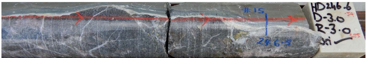
Fig 29 Hole 15, 246.6m. Top argillised andesite dyke in contact with diorite bottom
