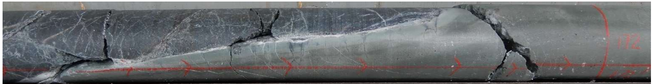
Fig 28 Hole 15, 172m. RHS argillised andesite dyke in contact with diorite LHS
