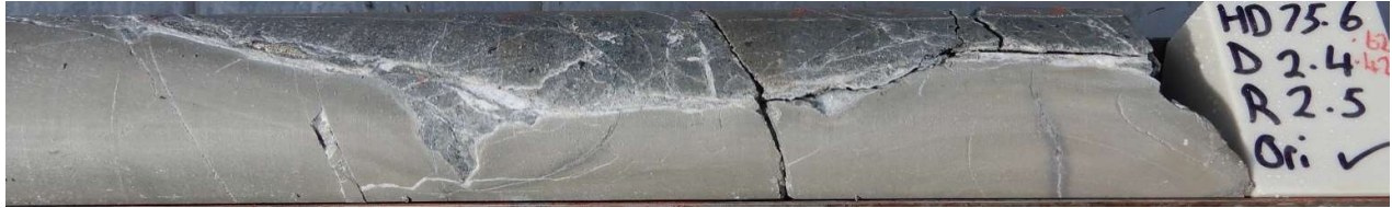
Fig 27 Hole 15, 75.6m Bottom shows argillised andesite dyke running down core in contact with diorite (top)
