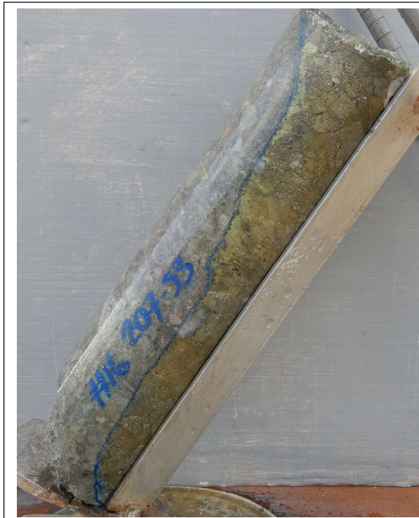
Fig 8 .Hole #16 , oriented in core oriented frame, hole drilling to south, inclined at 55.7degrees ,view looking west. LHS: 207.5m : semi-massive sulphide vein cutting sericitic, infill breccia. 207m to 208m : 1m @ 3.95% Cu, 0.62 g/t Au, 68.7 g/t Ag, 9.89% S. Vein strikes east west ( 070 mag) , dipping south at -68 degrees. (Dip direction = 160 mag).RHS :210m : Infill hydrothermal breccia . 210m to 211m: 1m 2.74% Cu, 0.43 g/t Au,71.6 g/t Ag, 4.41% S.
