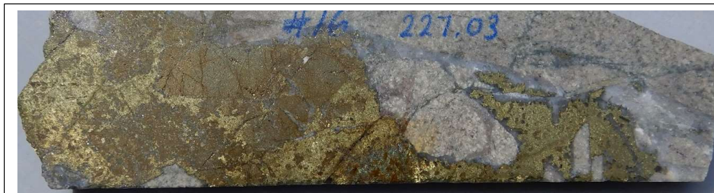
Fig 7 Bottom 227.03m 227m to 228m : 1m @ 2.56% Cu, 0.41 g/t Au, 42.7 g/t Ag.
