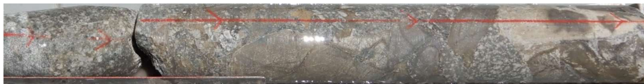
Fig 13. Hole 16, 420.5m, Close packed, clast supported bleached, polymict breccia with clasts of fine grained hornfels, altered diorite (both porphyritic and even grained). Minor infill rock-flour, pyrite, quartz. 420m-421m : Low sulphide.
