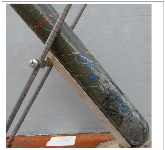
Fig 10 .Hole #16 , oriented in CoF, hole drilling to south, inclined at -53 degrees view looking east. LHS 294.9m : uphole hydrothermal breccia in contact with green, fine grained (post mineral) andesite. RHS 300.7m, green andesite dyke, in contact downhole with hydrothermal breccia . Dyke is trending east west , dipping steeply to south , measured as dipping -80 degrees towards 195 at top contact (LHS) and -80 degrees dip direction 190 at bottom contact (RHS). CAE Hole #16 is at right angles to Hole 15 which unfortunately drilled west to east ,in and out of these relatively thin andesite dykes which have true thicknesses in the range 0.2m to 5m.
