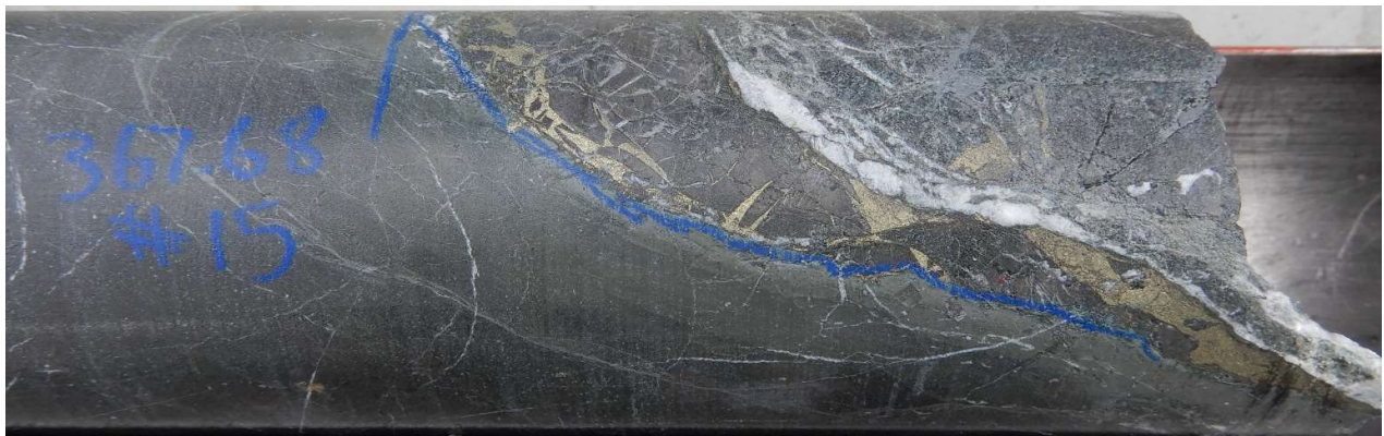
Fig 31 Hole 15, 367.68m. Top pyritic hornfels infill breccia (top) low angle contact with argillised andesite dyke (bottom).
