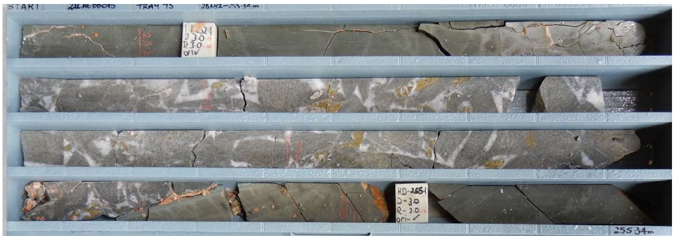
Fig 26 Photo half HQ core Hydrothermal infill breccia wedged between post mineral andesite dyke (green even grained). Hole #15, 253m-255m : 2m @ 1.06% Cu,0.15 g/t Au, 19.4 g/t Ag.
