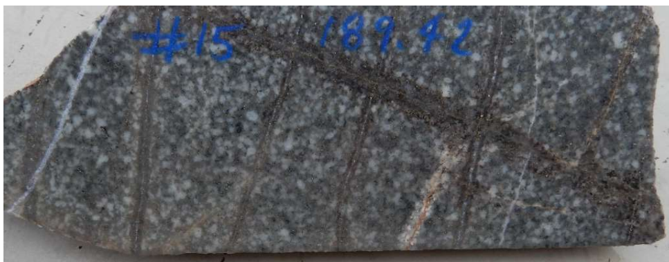
Fig 21. Hole #15, 189.9m Photo HQ Core fine sheeted quartz sulphide veins with alteration selvages, cutting earlier “porphyry-style” veins within crowded porphyry.
