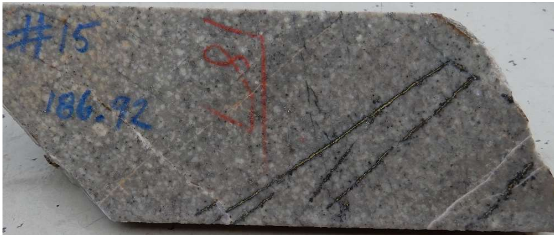
Fig 20. Hole 15, 186.9m. Photo half HQ Core fine sheeted chalcopyrite veins cutting sericite altered diorite crowded porphyry.
