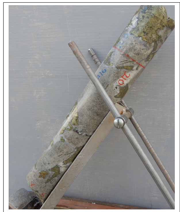
Fig 8 .Hole #16 , oriented in core oriented frame, hole drilling to south, inclined at 55.7degrees ,view looking west. LHS: 207.5m : semi-massive sulphide vein cutting sericitic, infill breccia. 207m to 208m : 1m @ 3.95% Cu, 0.62 g/t Au, 68.7 g/t Ag, 9.89% S. Vein strikes east west ( 070 mag) , dipping south at -68 degrees. (Dip direction = 160 mag).RHS :210m : Infill hydrothermal breccia . 210m to 211m: 1m 2.74% Cu, 0.43 g/t Au,71.6 g/t Ag, 4.41% S.
