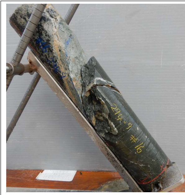
Fig 10 .Hole #16 , oriented in CoF, hole drilling to south, inclined at -53 degrees view looking east. LHS 294.9m : uphole hydrothermal breccia in contact with green, fine grained (post mineral) andesite. RHS 300.7m, green andesite dyke, in contact downhole with hydrothermal breccia . Dyke is trending east west , dipping steeply to south , measured as dipping -80 degrees towards 195 at top contact (LHS) and -80 degrees dip direction 190 at bottom contact (RHS). CAE Hole #16 is at right angles to Hole 15 which unfortunately drilled west to east ,in and out of these relatively thin andesite dykes which have true thicknesses in the range 0.2m to 5m.
