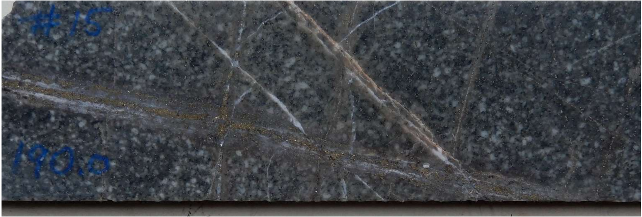
Fig 22 Hole #14, 190.0m. Photo half HQ core, multi-directional quartz sulphide vein stockwork with alteration selvages, typical “porphyry-style” veins cutting diorite.
