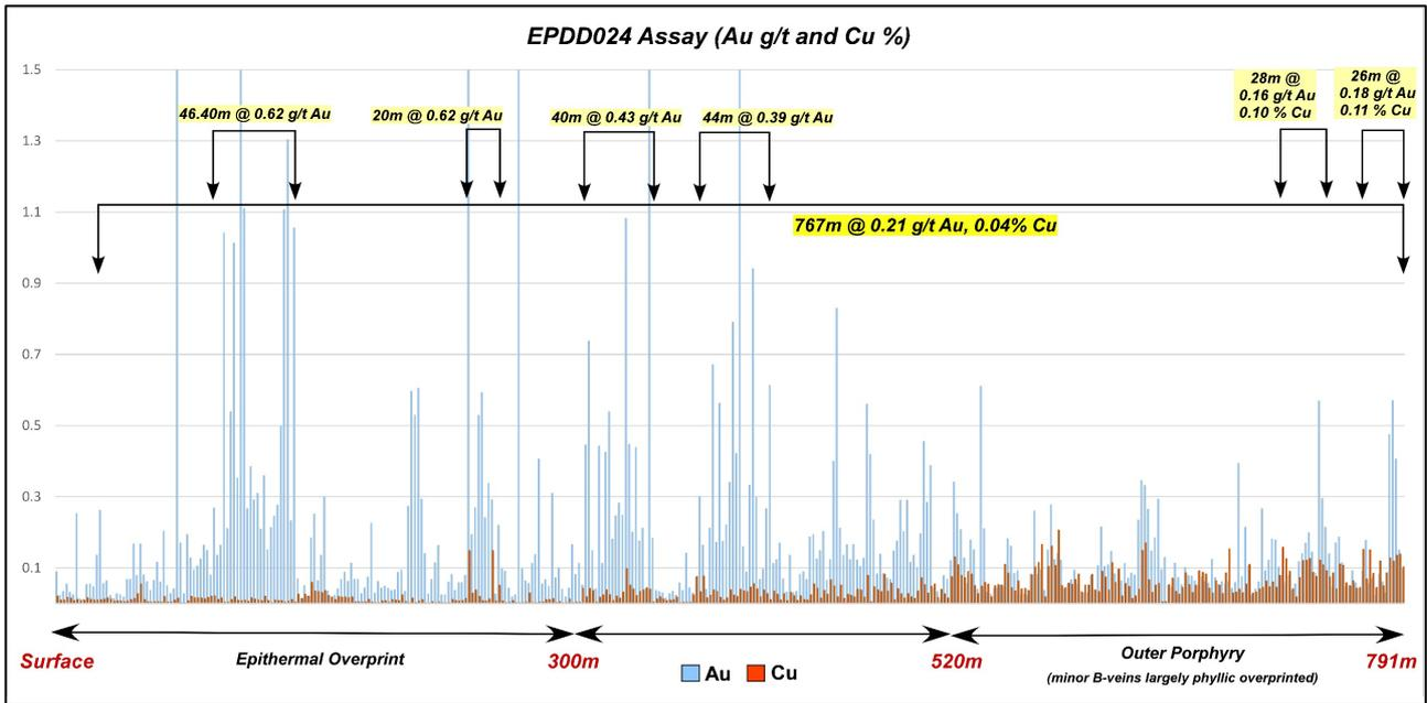
Figure 4: Drill hole EPDD024 down hole assay plot clearly showing upper-level epithermal overprint dominated by gold, and lower copper-gold porphyry signature.
