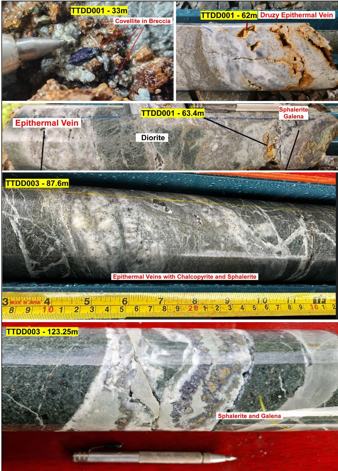
Figure 6: Drill core from Tituana drilling showing epithermal vein systems and mineralisation.
