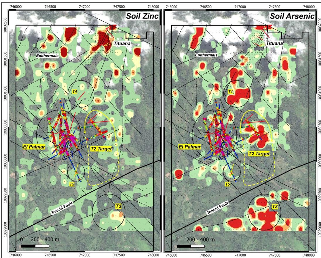
Figure 5: Extent of soil sampling at El Palmar (fine black dots), soil zinc anomalies that define epithermal targets in the northern part of the concession, and soil arsenic anomalies that define both epithermal targets and the locus of underlying porphyry targets at T2 plus T3 and T4 (both untested by drilling). The outline of the T2 target has expanded
