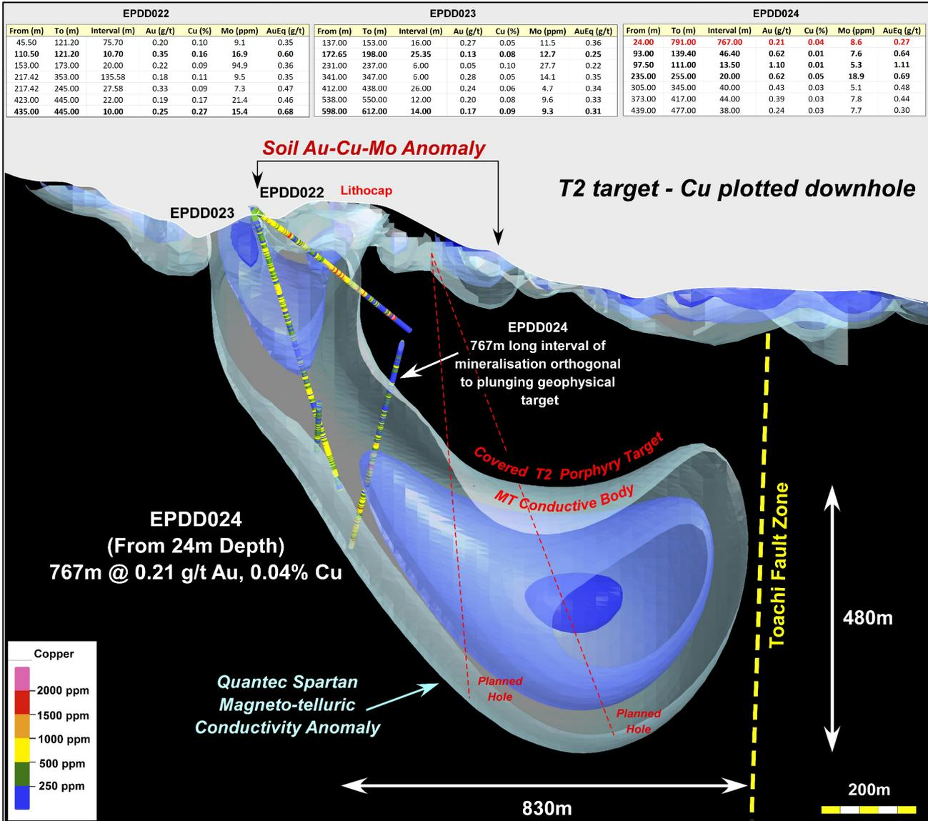
**Figure 1:** North-South section through the T2 target, showing outcropping porphyry stockwork near the collar of holes EPDD023/024 in the area of anomalous copper, gold and molybdenum in soils and coincident with a large area of weakly conductive material. This conductive body expands and strengthens southward and extends 800m south of the 767m-long intersection in hole EPDD024 that cuts the conductive body orthogonally. Two drill holes are planned and shown on section.
