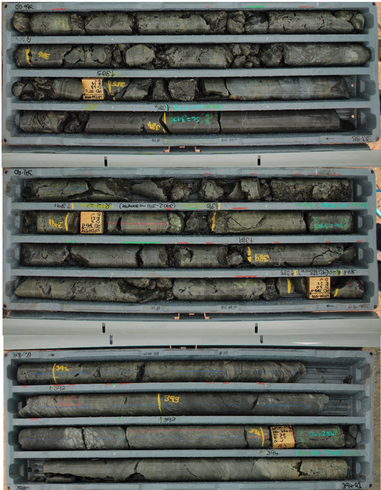
Figures 10: Drill core from Amy hole WFDH558, showing massive pyrite – chalcopyrite, and galena – sphalerite mineralisation from PY3
