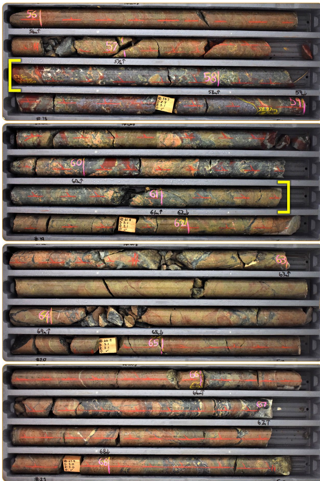
Figure 8. Drill core trays from MM008 showing quartz-chalcedony-adularia veins +/- galena, sphalerite and hematite, including zone of semi-massive (yellow brackets) galena-sphalerite-hematite-chlorite breccia hosting rounded chalcedony and quartz-chalcedony-adularia vein and breccia clasts within hematite-sericite altered rhyodacite tuff.
