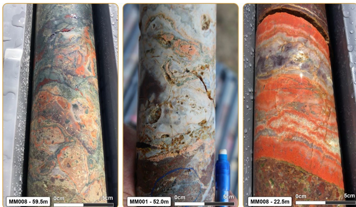
Figure 1. Hole MM008 and MM001 showing low sulphidation epithermal textured veins (chalcedony-quartz-carbonate) and breccia (galena-sphalerite-hematite). Quartz and chalcedony is white to dark grey and rarely purple in colour, adularia is orange to salmon pink, hematite is red, sphalerite may be white, light green to yellow and galena is silver to grey in colour. Note Cautionary statement about visible observations on Page 2.
