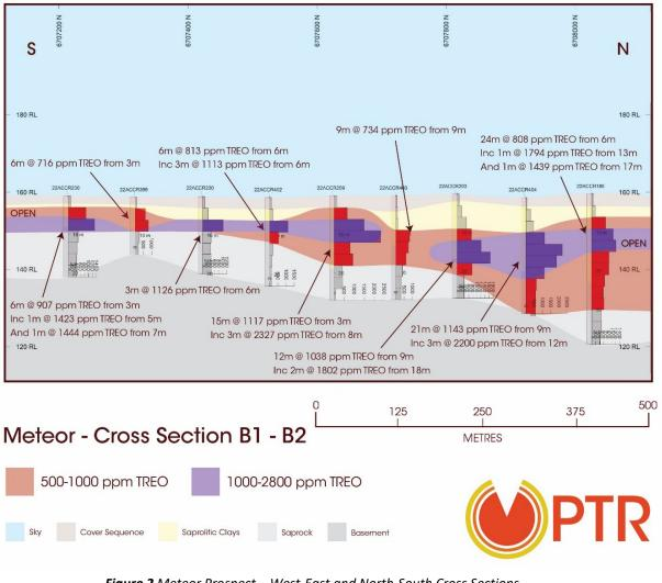
Figure 2 Meteor Prospect – West-East and North-South Cross Sections www.petratherm.com.au
