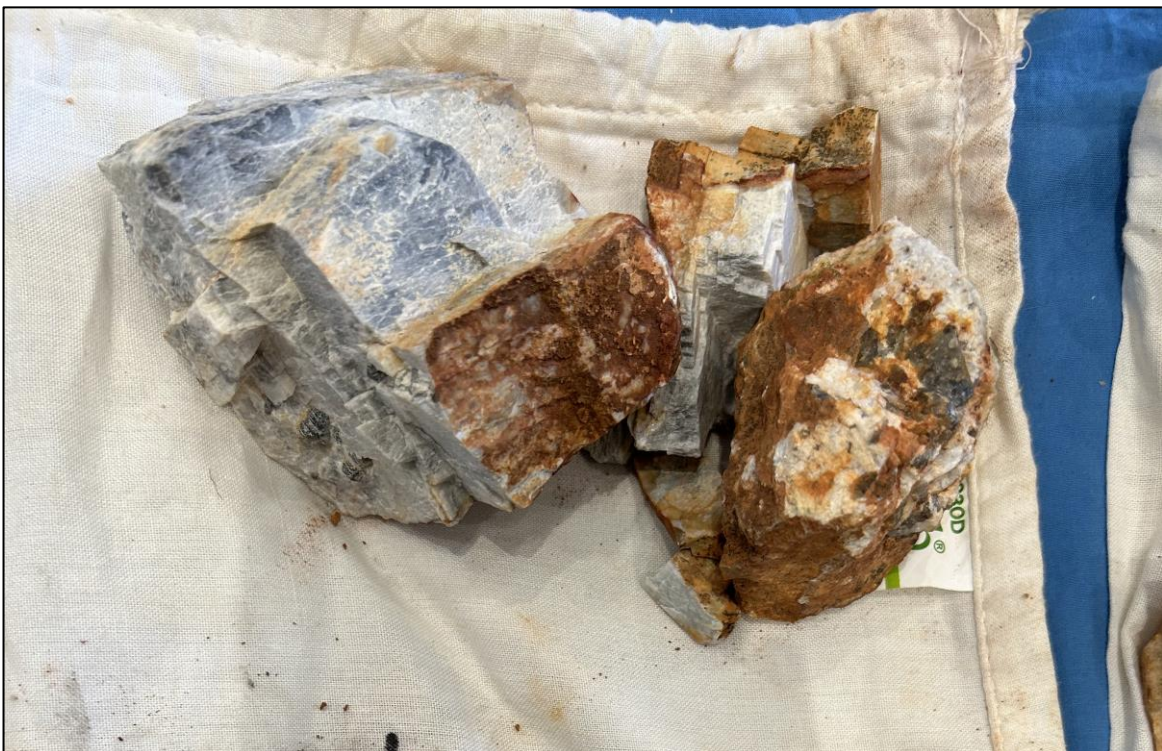
Figure 1 – Weathered pegmatite rock chip and MDK003b, dominated by microcline feldspar and heavily enriched in Rb. Image is approx. 20cm across.
