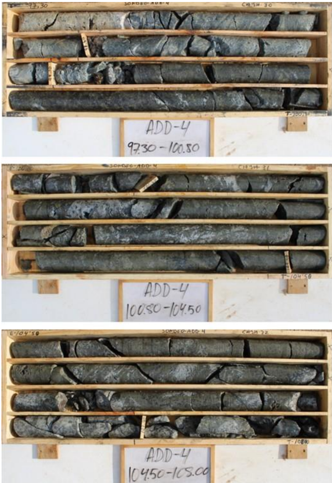
Figure 3 Drill hole ADD-04 core photos– Semi massive to massive sulphide mineralisation from 99.2-108.0m
