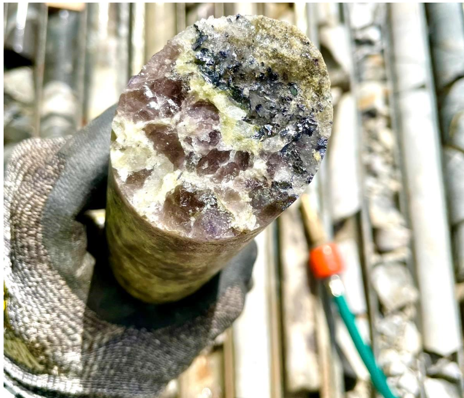
Figure 1. Coarse grained fluorite (purple) with wolframite (black) and molybdenite (silver) with quartz ± carbonate ± sericite
