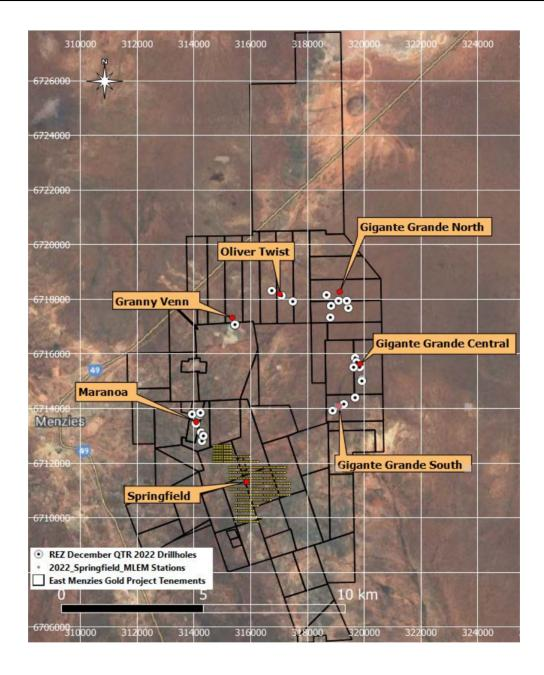
The MLEM over the Springfield Prospect targeted a highly altered sequence of komatiite basement rocks which are prospective for disseminated and massive Ni-Fe sulphides. A total of 685 stations distributed along 25 lines @ 200m line spacing were originally planned in a series of east west lines. Due to difficult terrain and time constraints the program was modified to include only 15 higher priority lines.
